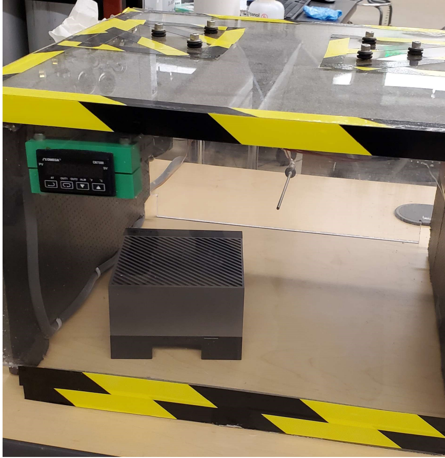
Figure 6.1 The heat generation unit used for testing performance of the Orin at different external temperatures.
