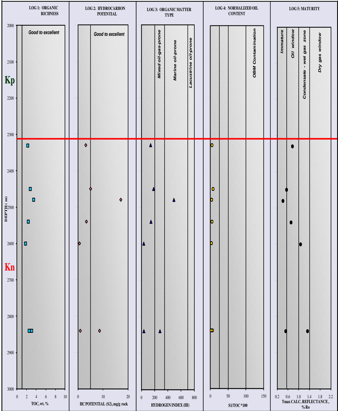
Figure 4.9 Geochemical Log for the samples tested for Government 1. TOC (wt. %), S2 (mg HC/g rock), HI, S1/TOC*100, and Tmax calculated vitrinite reflectance are presented. Cuttings from Government 1 were sampled on 30-240 feet intervals, with a total of 6 samples, from 2330 to 2840 feet. Formations are indicated by labels; Kc (Carlie), Kf (Frontier), Kn (Niobrara) and Kp (Pierre).
