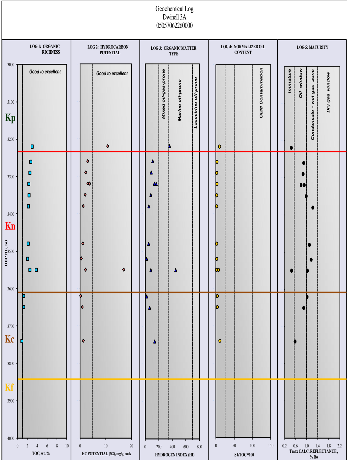
Figure 4.3 Geochemical Log for the samples tested for Dwinell 3A. TOC (wt. %), S2 (mg HC/g rock), HI, S1/TOC*100, and Tmax calculated vitrinite reflectance are presented. Cuttings from Dwinell 3A were sampled on about 30 feet intervals, with a total of 12 samples, from 3220 to 3740 feet. Formations are indicated by labels; Kc (Carilie), Kf (Frontier), Kn (Niobrara) and Kp (Pierre).
