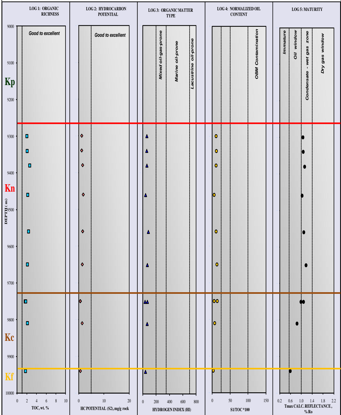
Figure 4.13 Geochemical Log for the samples tested for Meyring 41-10. TOC (wt. %), S2 (mg HC/g rock), HI, S1/TOC*100, and Tmax calculated vitrinite reflectance are presented. Cuttings from Meyring 41-10 were sampled on about 30 foot intervals, with a total of 9 samples, from 9300 to 9940 feet. Formations are indicated by labels; Kc (Carilie), Kf (Frontier), Kn (Niobrara) and Kp (Pierre).
