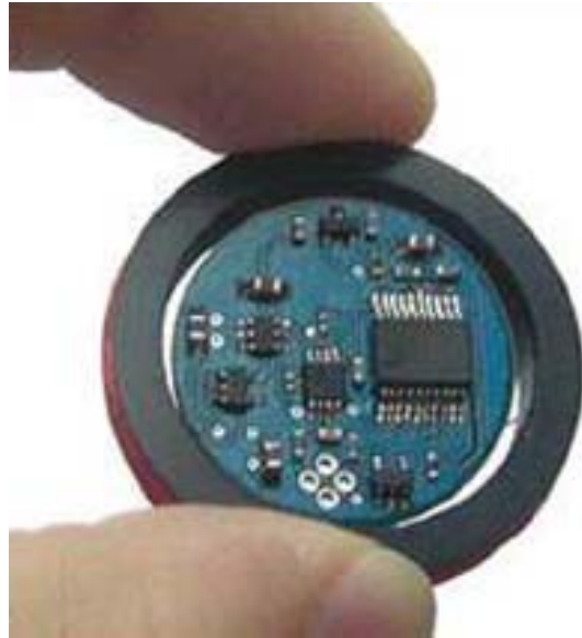
Figure 2.5: MicroStrain EmbedSense transceiver with induction coil.
