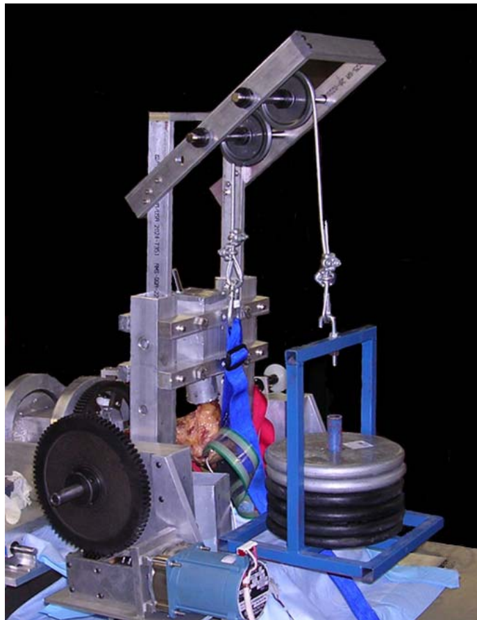
Figure 5.5: A leg specimen loaded into the knee testing apparatus. The applied load, pulley apparatus and attachment to the quadriceps are shown.
