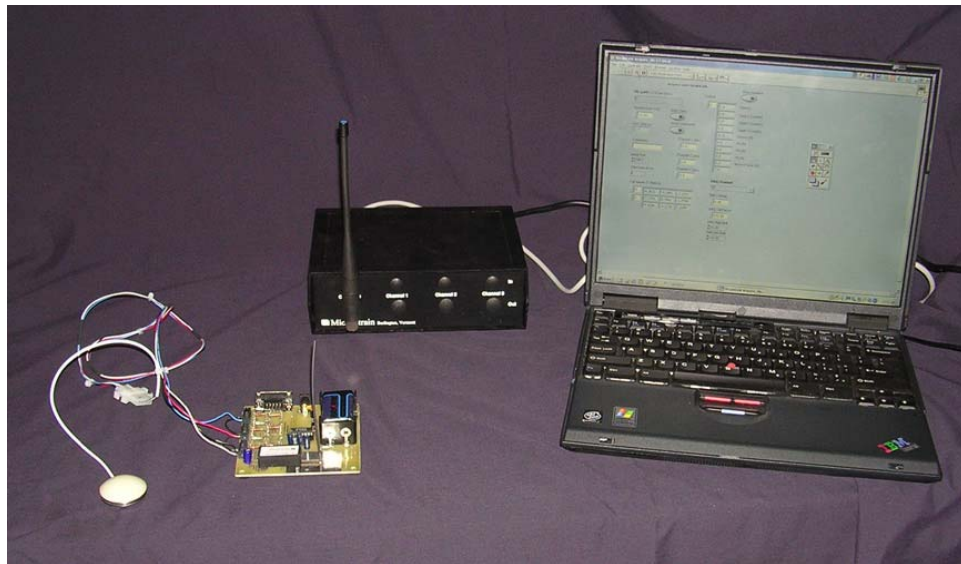
Figure 3.3: Wireless data acquisition system with StrainLink instrumentation.
