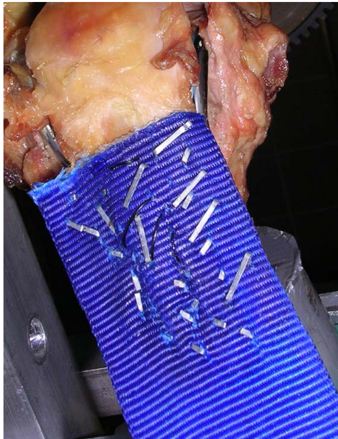
Figure 5.4: Attachment of the quadriceps tendon to the tubular webbing.
