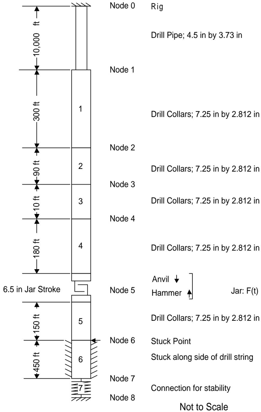
Figure 7-1: Case 1—Drill String Schematic
