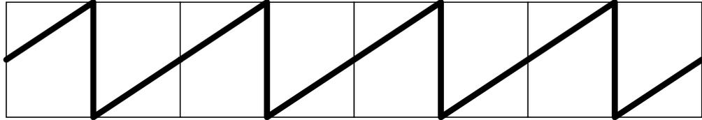
b) Endpoints in each time window do not match. Leakage will occur.
