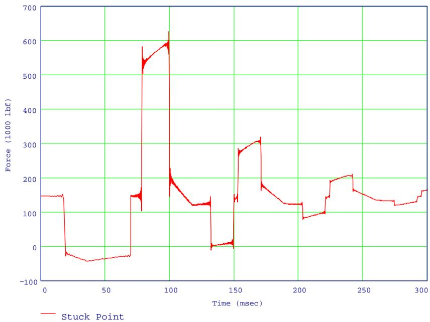
**Figure 7-13: Case 2—Forces at the Top of the Stuck Point**
