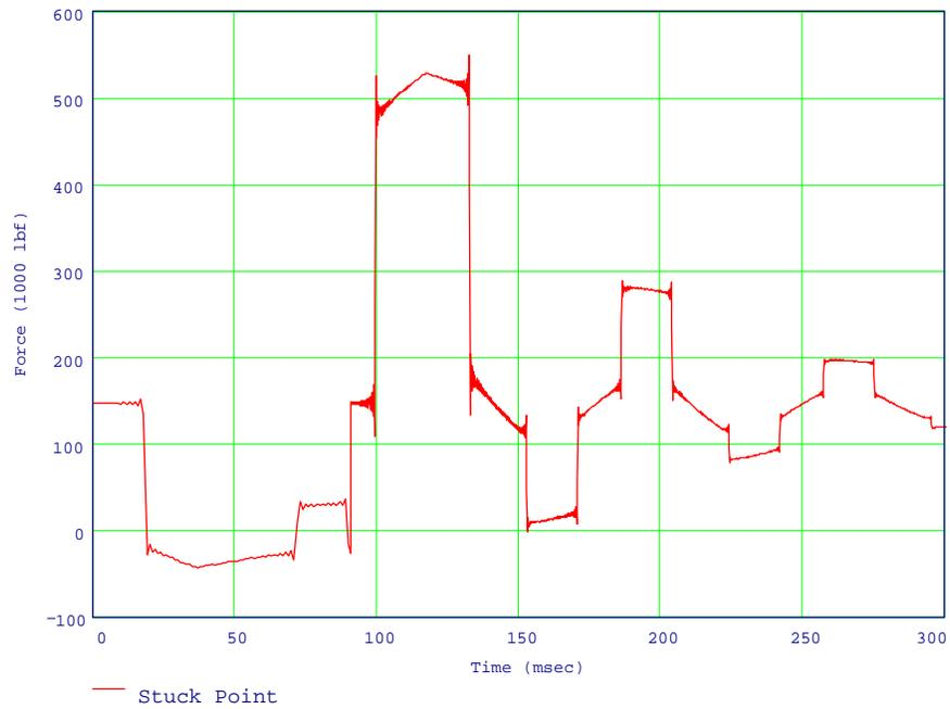
**Figure 7-19: Case 3—Forces at the Top of the Stuck Point**
