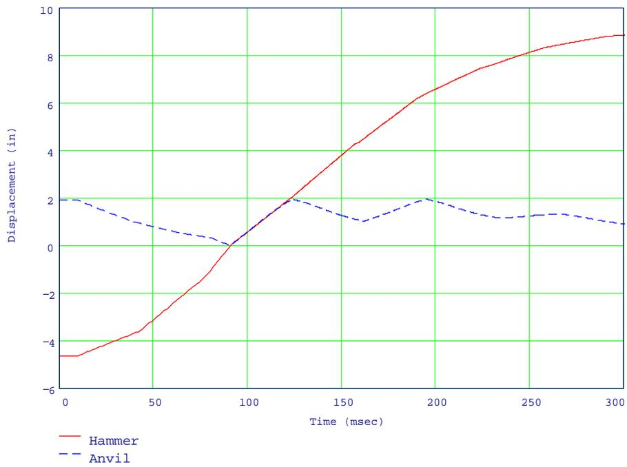
**Figure 7-15: Case 3—Displacement of Hammer and Anvil**
