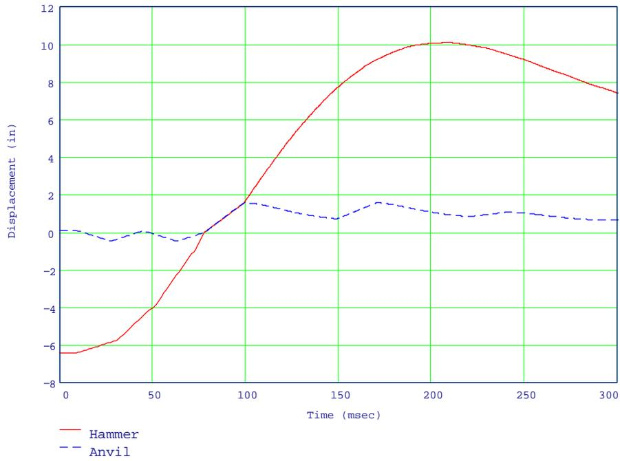
Figure 7-27: Case 5—Displacement of Hammer and Anvil
