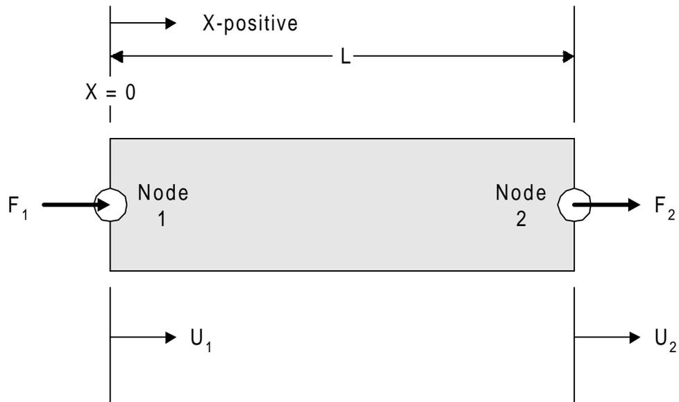
**Figure 4-3: Two Noded Axial Finite Element**
