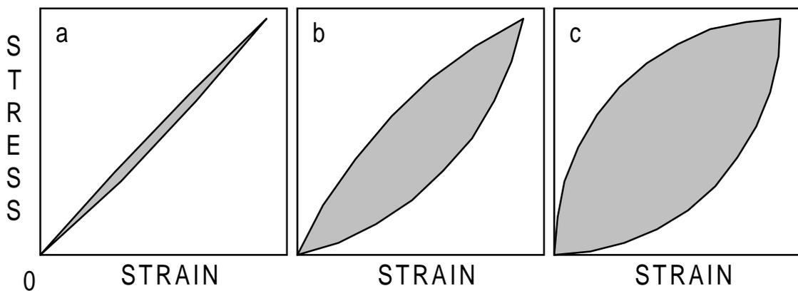
**Figure 4-1: Examples of Hysteretic Damping**
