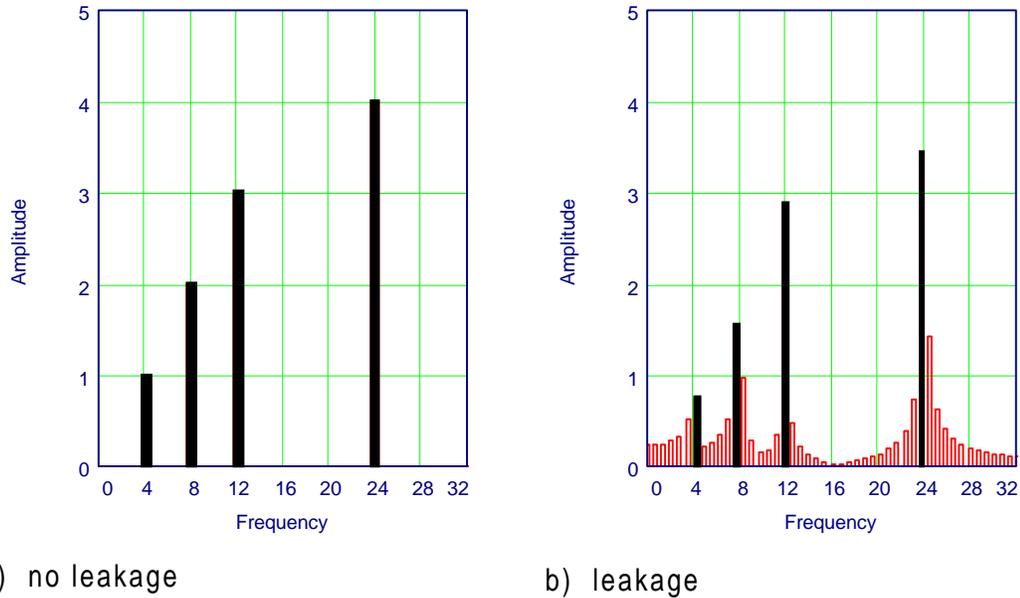
**Figure 3-9: Example of Leakage**
