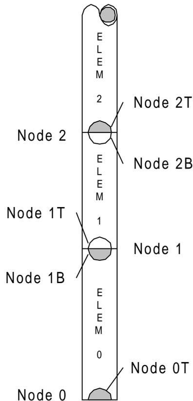
**Figure 5-3: Example Node and Element Numbering**
