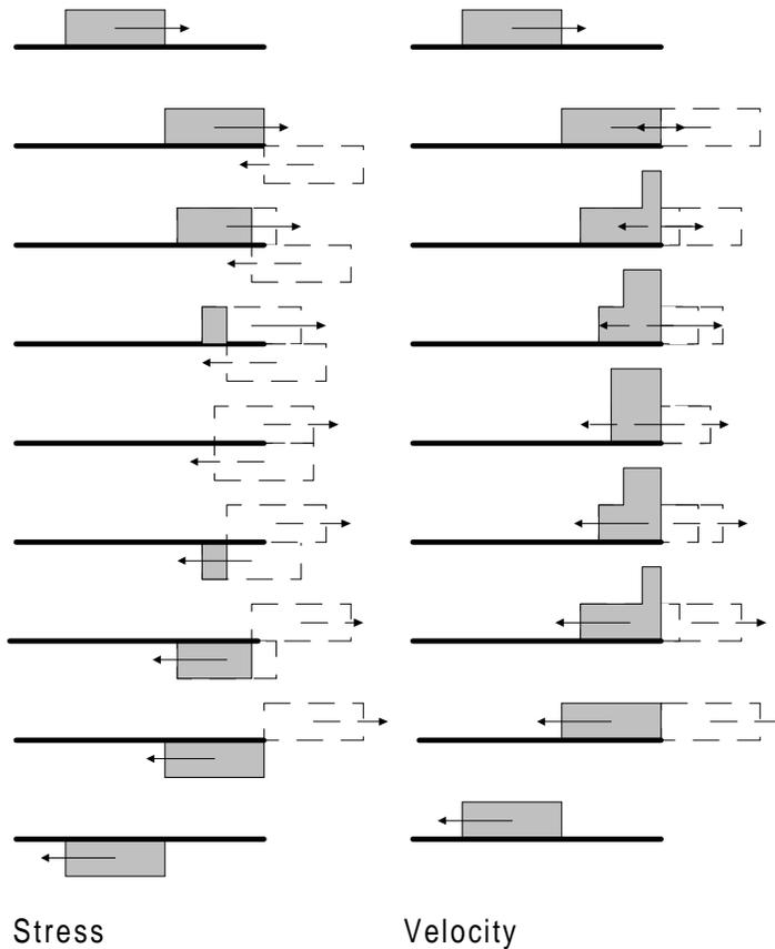
**Figure 5-2: Free End Boundary Conditions**
