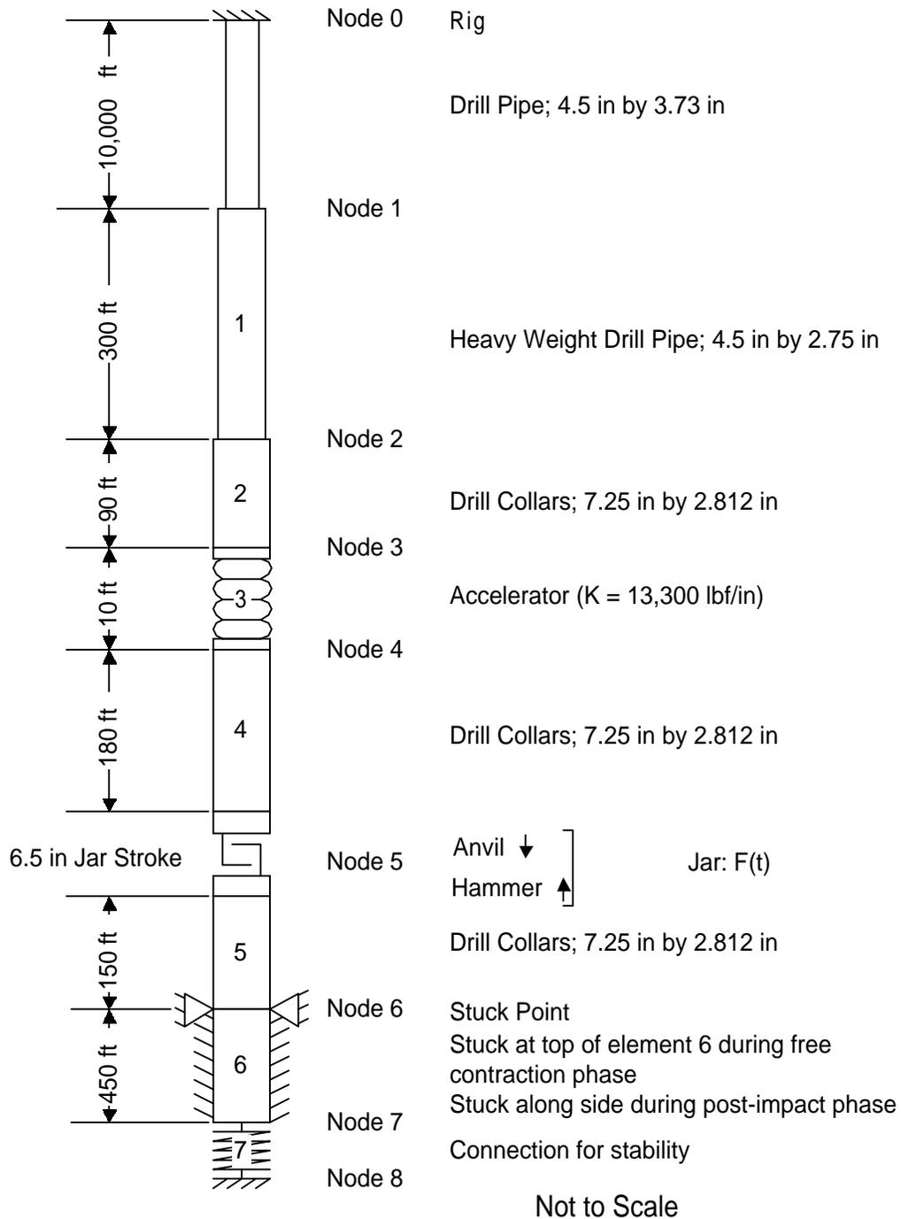
Figure 7-26: Case 5—Drill String Schematic
