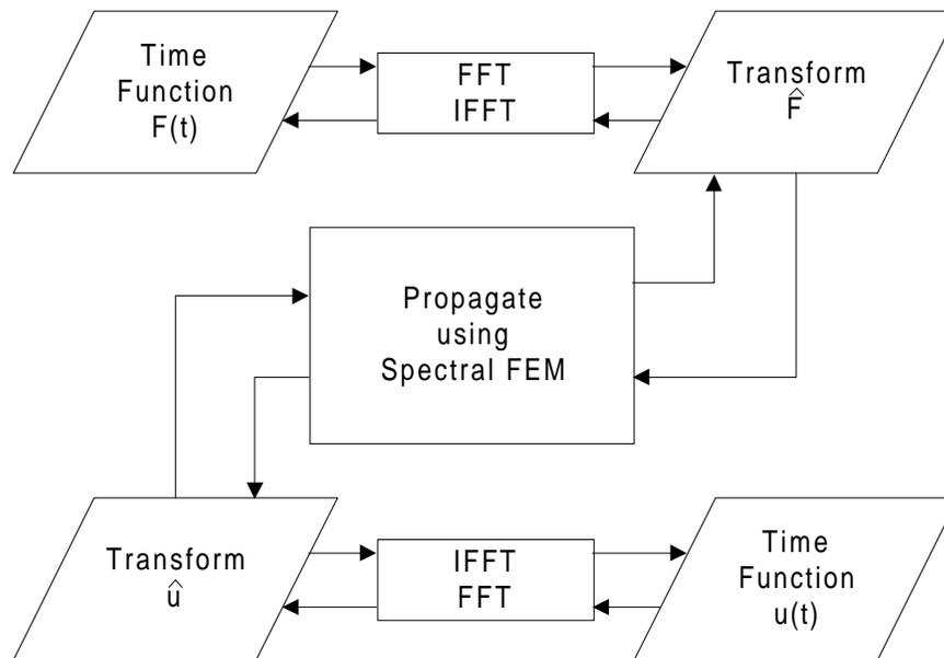
**Figure 4-5: Spectral Analysis Procedure**
