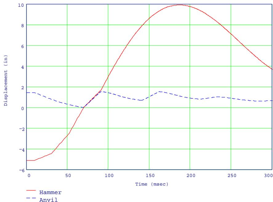
**Figure 7-9: Case 2—Displacement of Hammer and Anvil**
