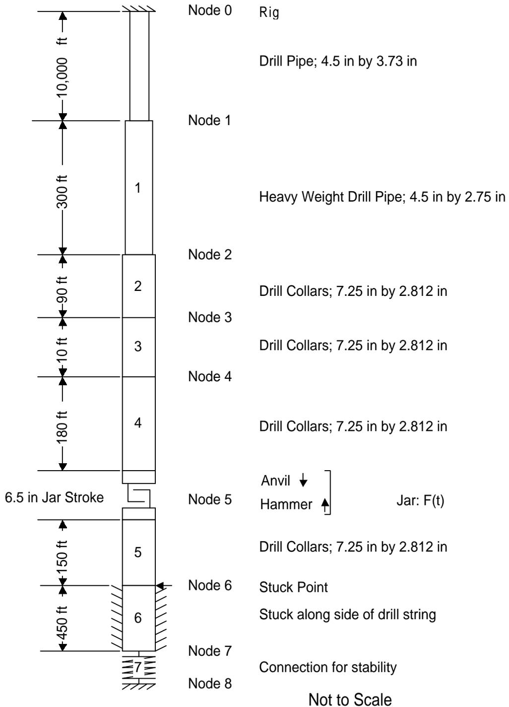
Figure 7-14: Case 3—Drill String Schematic
