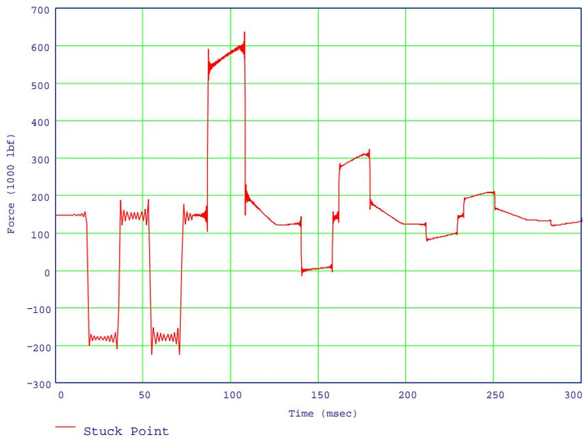
Figure 7-31: Case 5—Forces at the Top of the Stuck Point
