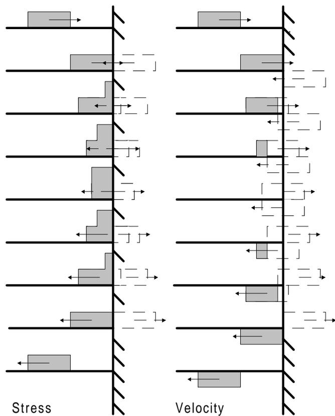
**Figure 5-1: Fixed End Boundary Conditions**
