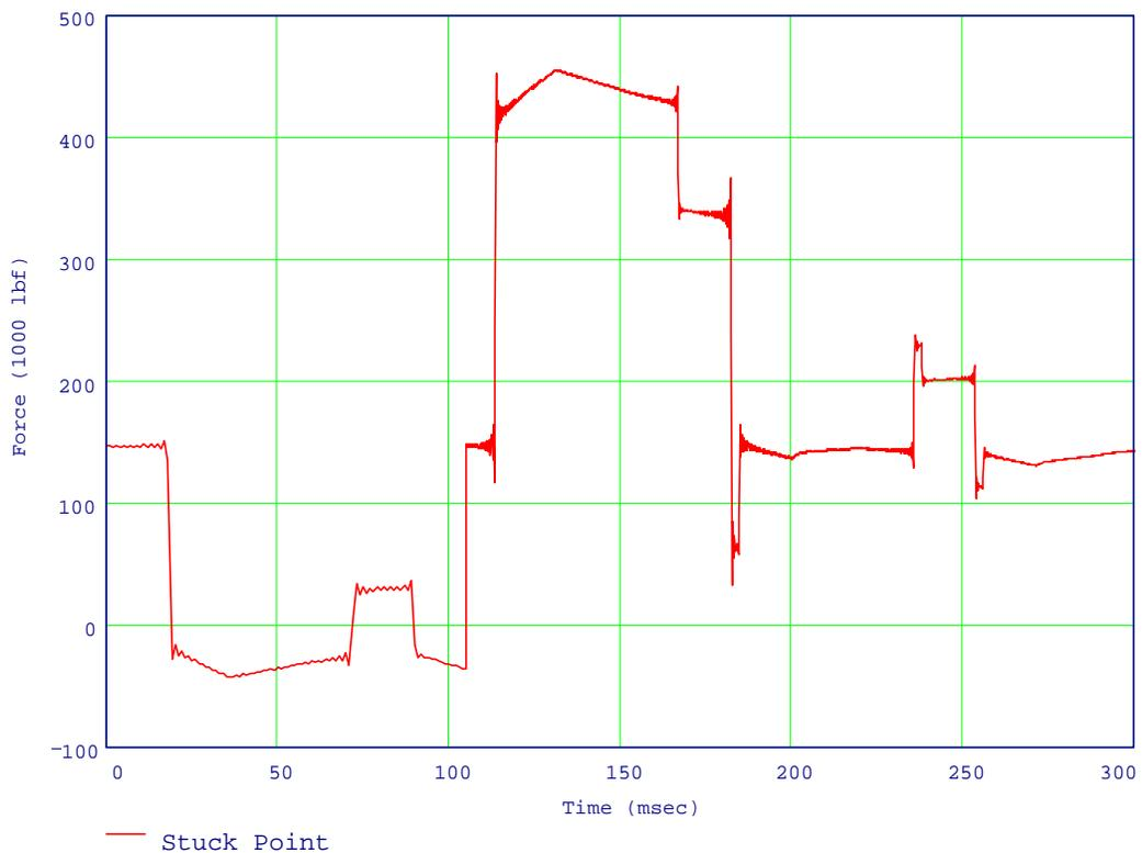
**Figure 7-7: Case 1—Forces at the Top of the Stuck Point**
