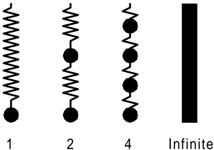
lumped at the nodes is essentially converting the pipe into a the system into a series of point masses and massless springs. (See Figure 3-2.) This means that there will be a finite number of natural frequencies rather than the actual infinite
