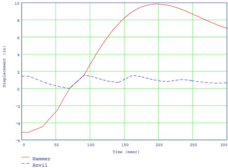
Figure 7-21: Case 4—Displacement of Hammer and Anvil
