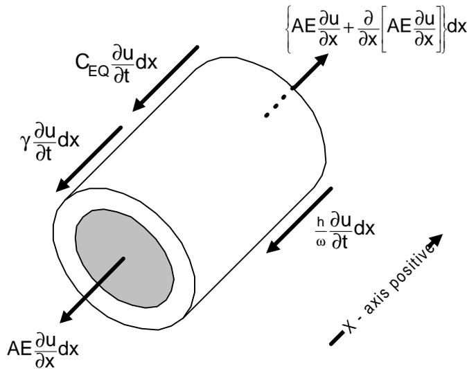
be inclined as long as it is straight. The various dynamic forces acting on a differential element are shown in Figure 4.2.
