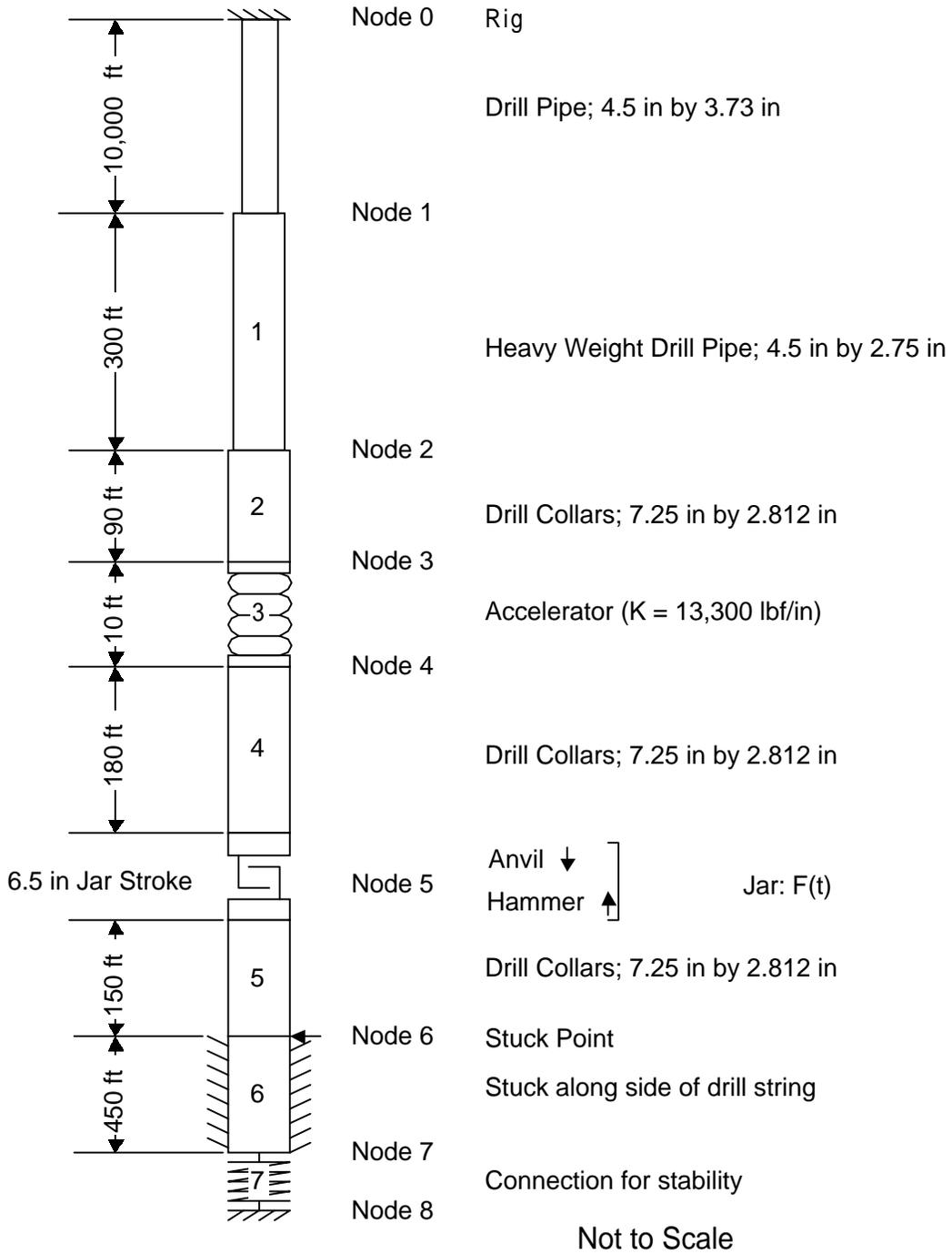
Figure 7-20: Case 4—Drill String Schematic
