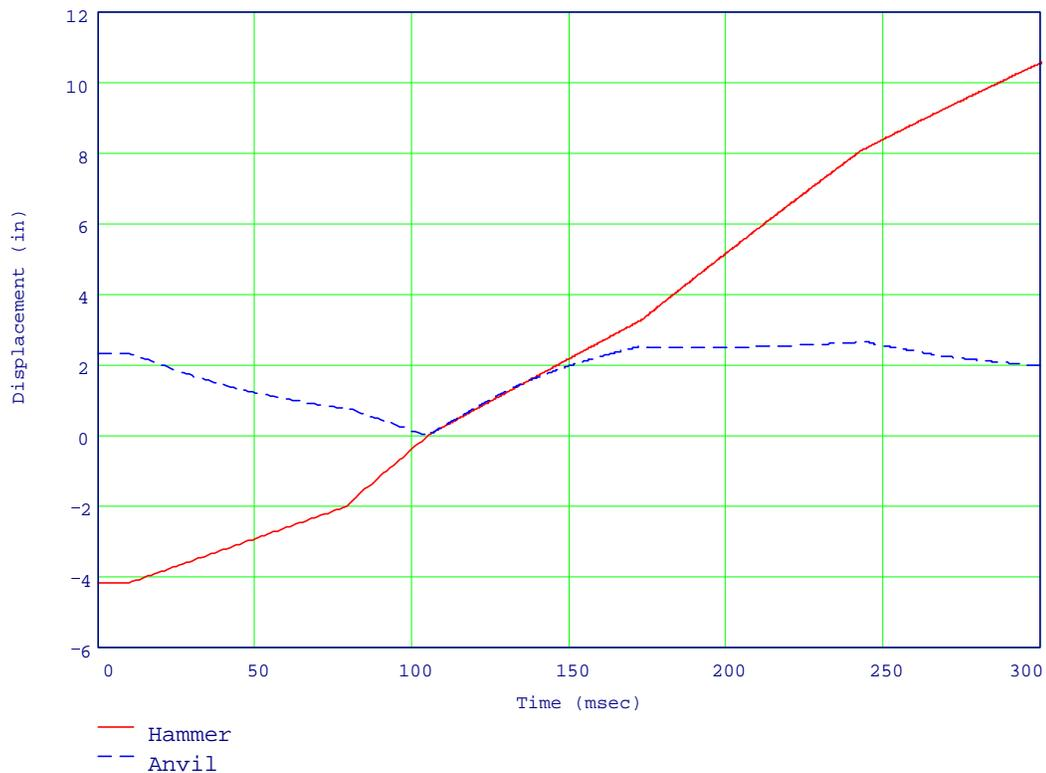
**Figure 7-3: Case 1—Displacement of Hammer and Anvil**
