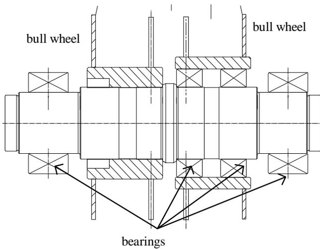
Fig. 2 Axle for bull wheels of ropeway, (axle rotates, one wheel fixed)
