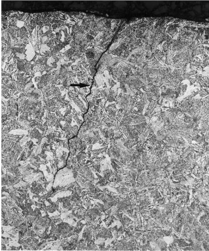
Fig. 4 Crack initiated by fretting fatigue
