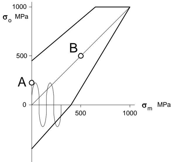
Fig. 9 Smith-diagram for fatigue strength of steel 42CrMo4
