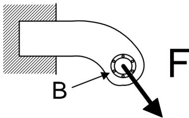
Fig. 7 Example of a structure loaded in tension with a force  $F$ , having a stress concentration at the hole  $B$  where the load is introduced
