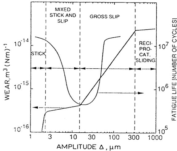
Fig. 5 Damage and slip (Vingsbo and Soederberg , 1988)
