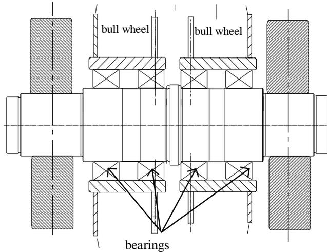
Fig. 8 Design with fixed axle and rotating bull wheels
