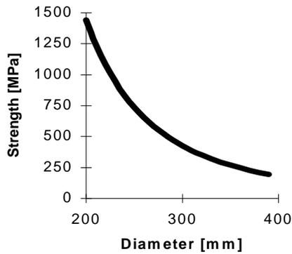
Fig. 6 Relation between strength and diameter of a shaft
