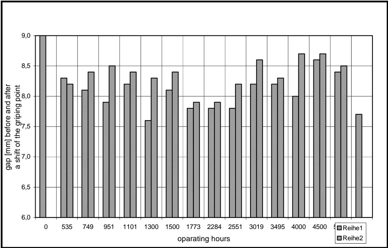
**Picture 5:** Readings of gaps at the grip, measured before (Reihe 1) and after (Reihe 2) a shift of the gripping point
