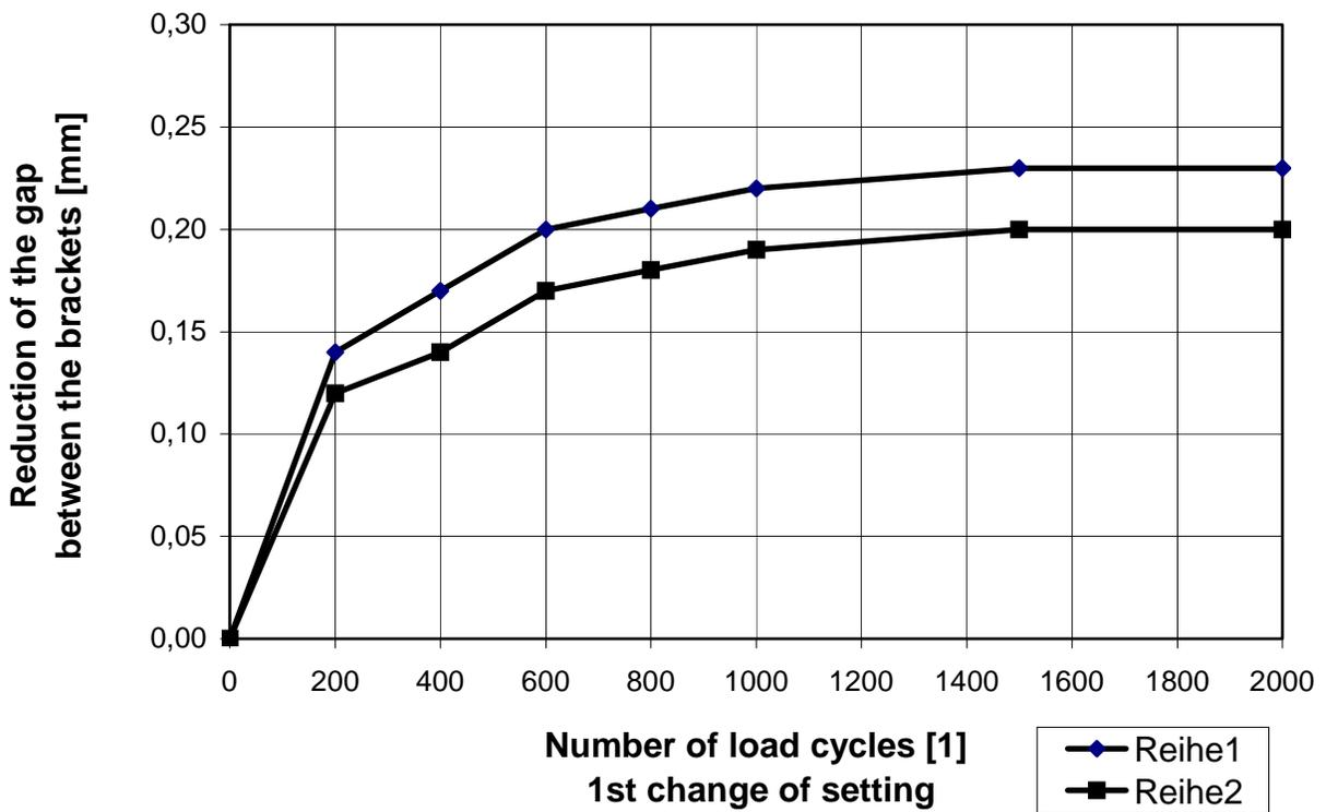
**Picture 2 and 3:** Wear on the padding according to the number of load cycles
