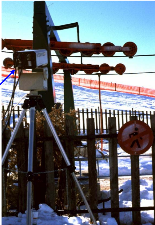
Fig. 1: Laser scanning vibrometer set-up and the sheave assembly analysed
