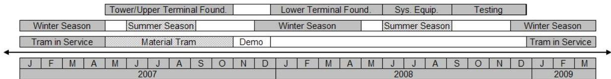
**Figure 5 - Tramway Construction Schedule**
