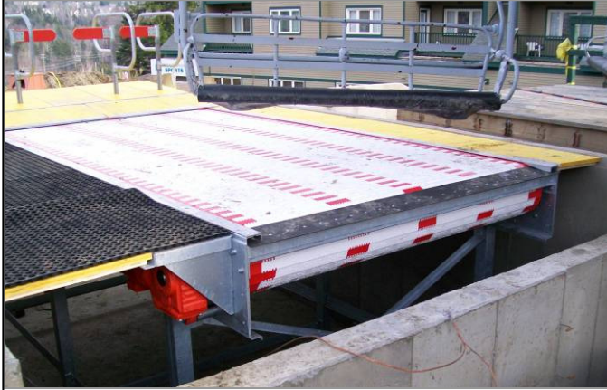
Mount Snow 2008 – Detachable – Deep pit without front load boards attached yet. Shows snow scrapper on front drum. Note center post of load gate removed for ADA access and lane markings on the carpet.
