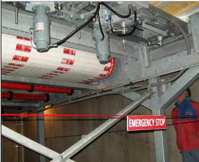
Mount Snow – 2008 – deep pit – drive motors for load gates – manual release levers on each motor.
