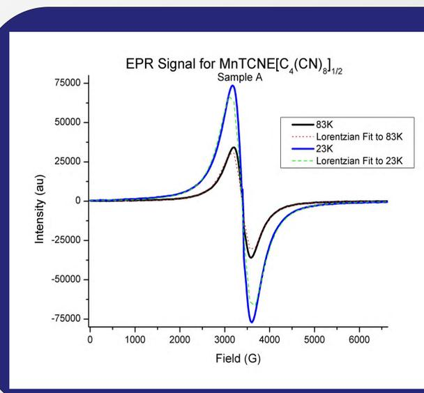
Figure 4. EPR lineshape for Sample A at 23 K and 83 K
