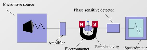
Figure 3. The diagram of an electron paramagnetic resonance system
