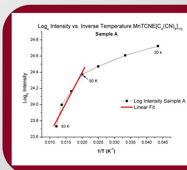
Figure 6. Logarithm of intensity versus inverse temperature from 30-83 K for Sample A
