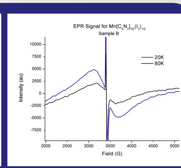
Figure 5. EPR lineshape for Sample B at 20 K and 80 K (Note: spikes are artifacts)
