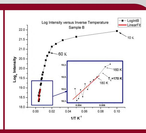
Figure 7. Logarithm of intensity versus inverse temperature from 10-260 K for Sample B
