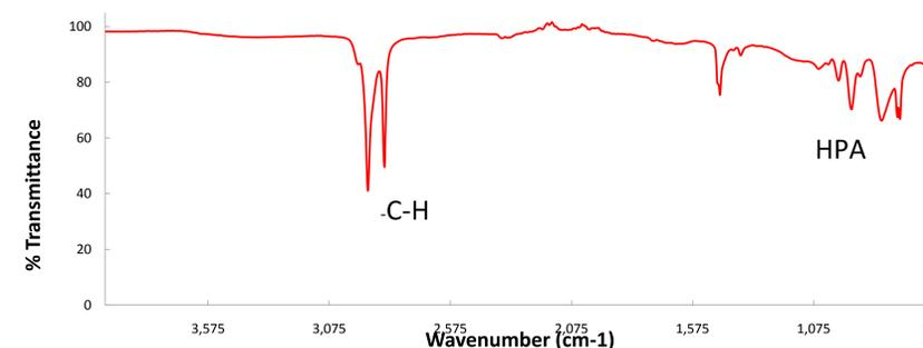
IR of HPA/ethylene co-monomer with polyethylene backbone. There are no carbon-carbon double bonds indicating that the polymerization did indeed occur yielding the desired polymer.
