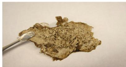
This is the first HPA-ethylene membrane made in the lab. After removing the co-monomer from the bomb the excess solvent was evaporated in a vacuum oven. To create a flexible backbone it was necessary to mix the co-monomer with solid polyethylene and dissolve in a like solvent creating a liquid. This liquid was evaporated off leaving a thick flexible membrane. Much needs to be improved upon to make the membrane more homogenous and thinner.
