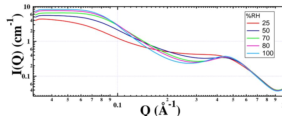
Above is data collected from the synchrotron at Argonne National lab, this trend shows how the morphology of the heteropolyacids in the membrane change as relative humidity changes
