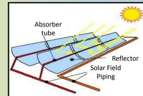
Figure 3: Parabolic trough
