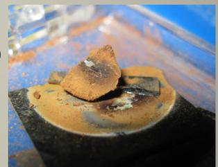
Bottom of a chunk of QD's charred by laser
