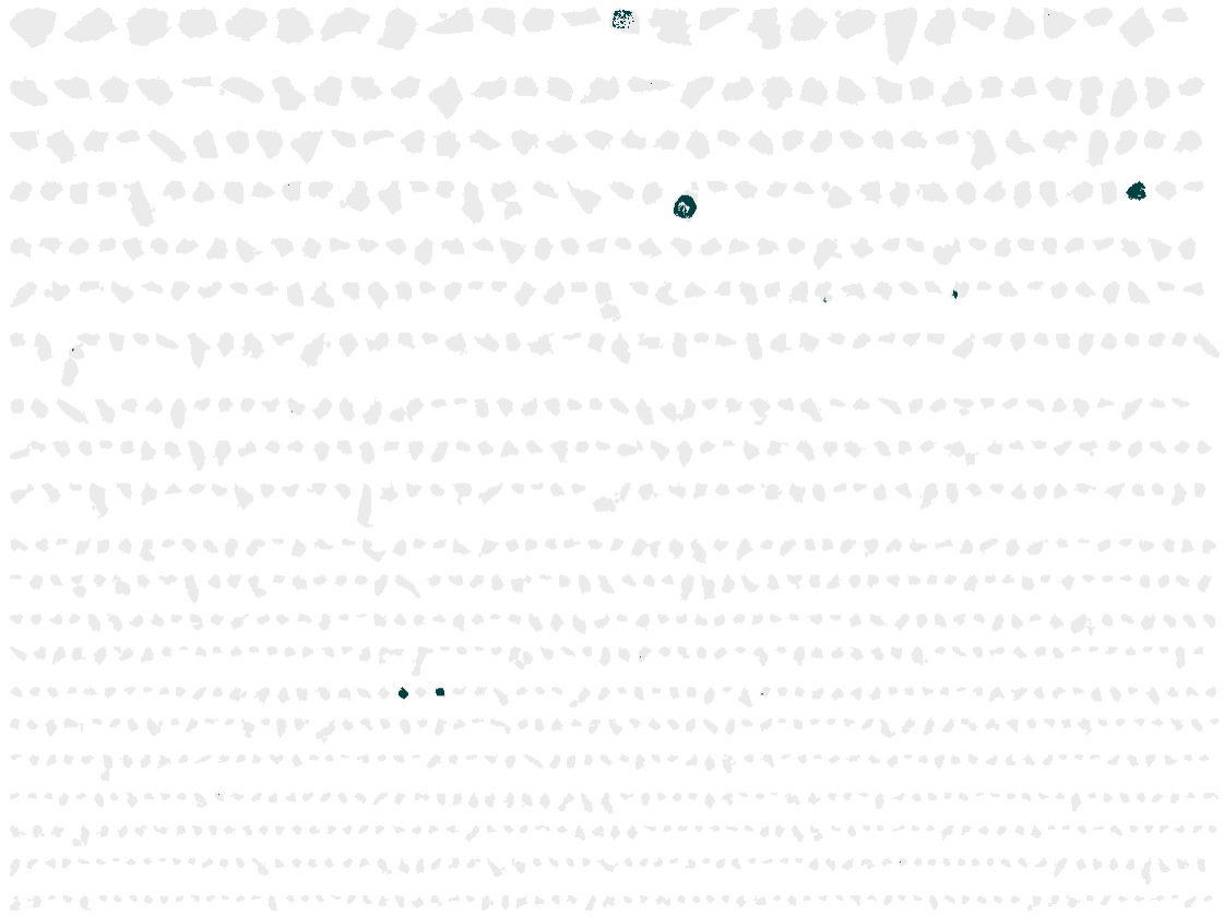
Figure 4-14: QEMSCAN Image of AlMn Phase
