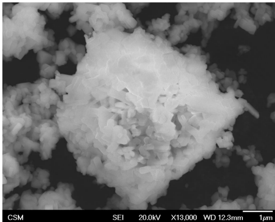
Figure D.1 Scanning electron microscope (SEM) image of the xenotime DyPO 4 sample powder. The powder has a sub-micron grain size (100-800 nm). The grains are often clustered into larger particles and exhibit the anisotropic shape expected of tetragonal crystals. This image was obtained using a JEOL 7000F SEM.
