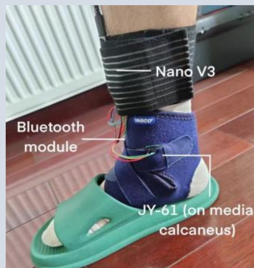
Figure 2: Ankle brace design using muscle stimulation [5]
