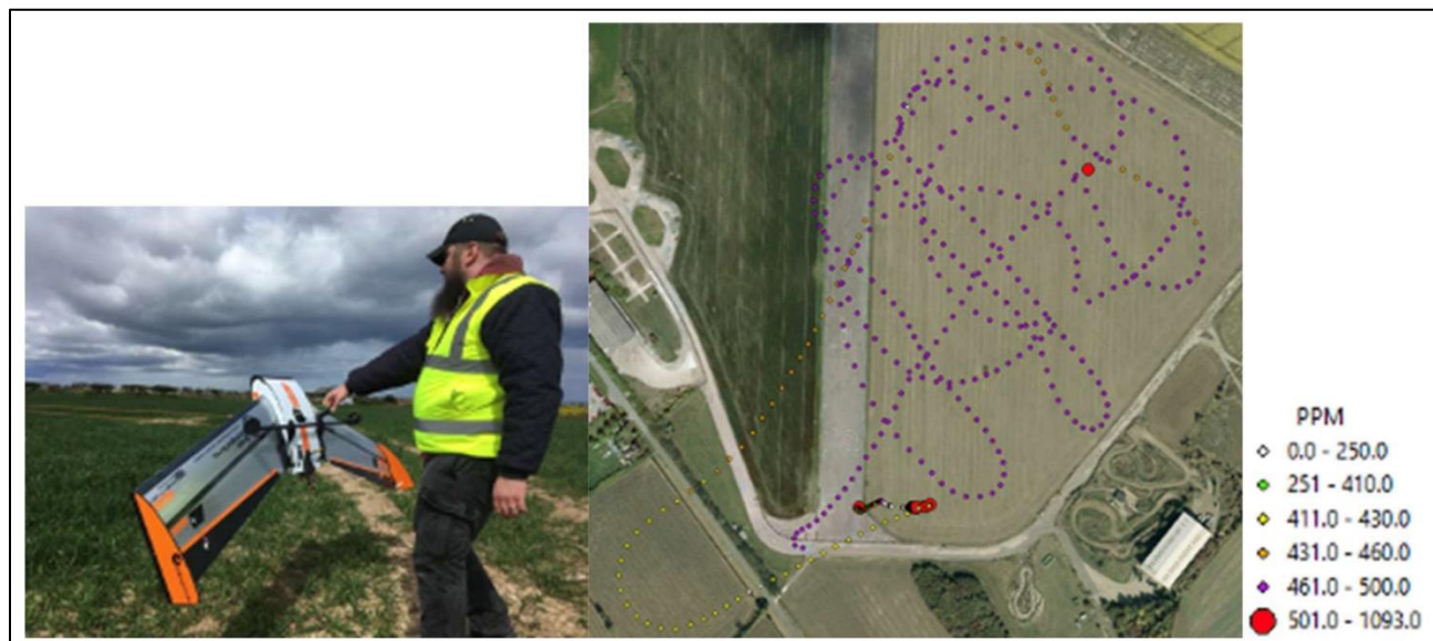
Figure 4: Left: Deployment of an atmospheric monitoring equipped drone. Right: Aerial image showing drone flight path, with each color-coded dot correlating to changing CO 2 levels. ( Image source )
