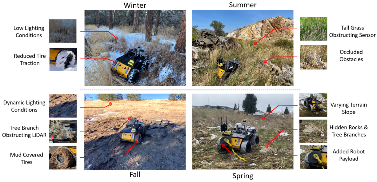
Figure 1.1 Motivating scenarios of robot lifelong adaptation in unstructured environments. When operating in these environments, mobile robots will encounter a complex combination of discrete or continuous and gradual or sudden changes in the environment and the robot itself. In addition, these environments have varying characteristics which cannot be modeled into the robot before deployment. Autonomous robots must, therefore, successfully adapt their perception, behaviors, and decision-making capabilities to achieve robust autonomy in such environments.
