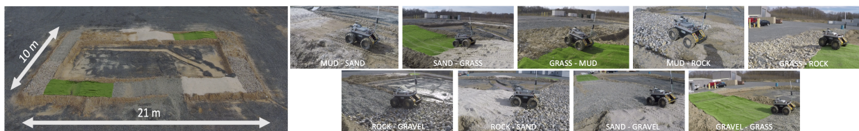
Figure 8.5 The off-road ground navigation circuit consists of different types of terrains (such as grass, gravel, large-rock, mud, and sand) as well as diverse terrain transitions. The size of the circuit is 10 x 21 meters with terrain slopes varying between 0 – 30°.
