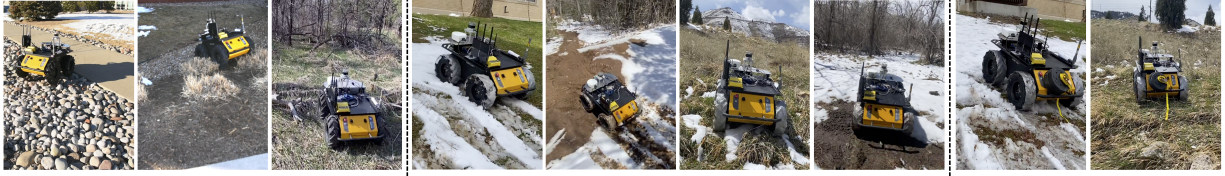
Figure 8.6 Various terrain tracks used to evaluate the self-reflection capability of the robot. From left to right: mixed terrain I (MT-I), mixed terrain II (MT-II), forest, reduced-traction snow-grass (RT-Snow-Grass), reduced-traction mud-snow (RT-Snow-Mud), reduced-traction hill (RT-Hill), reduced-traction forest (RT-Snow-Forest), reduced-traction payload snow-grass (RT-P-Snow-Grass) and reduced-traction payload hill terrain (RT-P-Hill).
