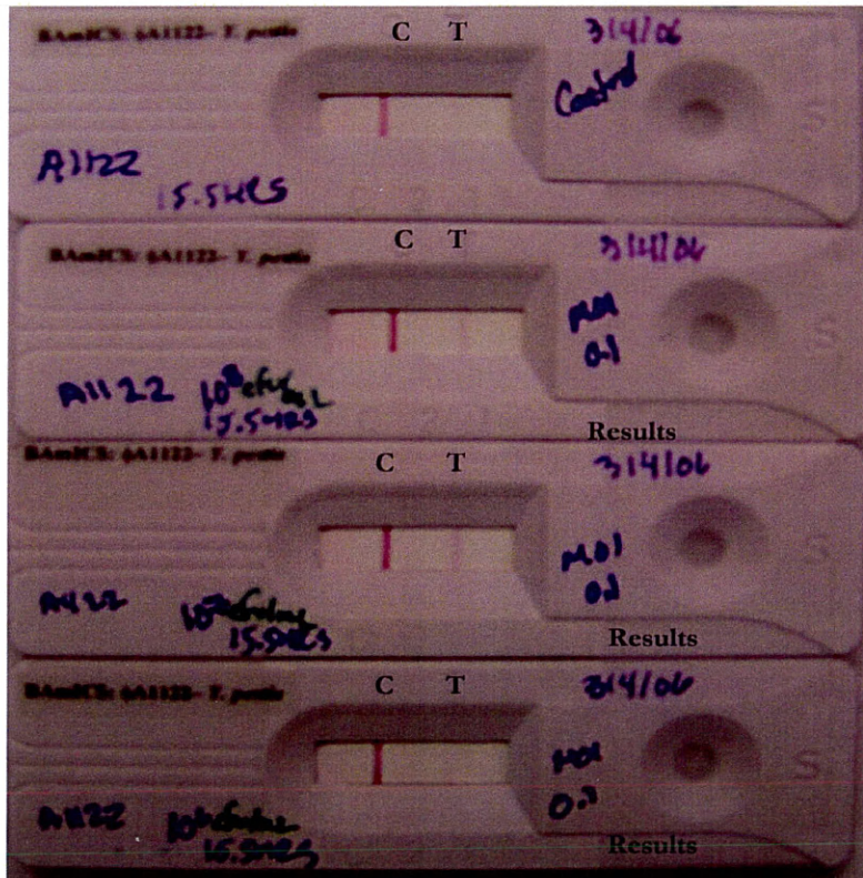
Figure 8.6 BAMICS sensitivity results. Sensitivity results of a 15.5 hour infectivity study with phage \phi A1122 and Y. pestis A1122. C and T indicate control and test lines respectively. Top detector shows bacteria only before initial infection, the subsequent three detectors show results of positive Y. pestis A1122 identification at 10^8 , 10^7 and 10^6 cfu/mL bacteria respectively.
