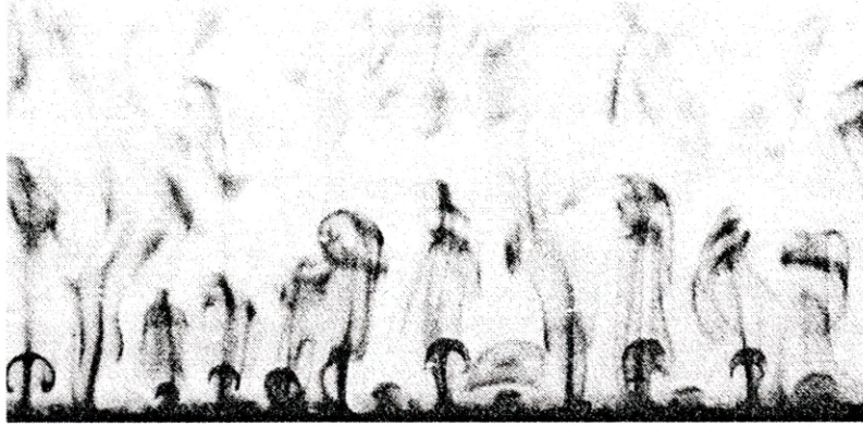
Figure 6.5. Rayleigh Taylor instability. Buoyant thermals rising from a heated plate. Image taken from An Album of Fluid Motion (Van Dyke, 1998). Experiment completed by Sparrow, Husar and Goldstein, 1970.
