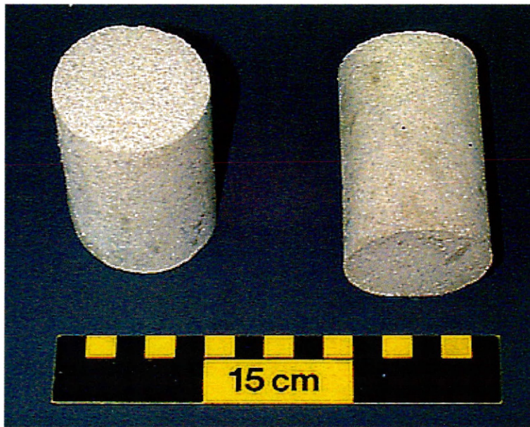
Figure 4.3 Photograph of two of the tetrahydrofuran-hydrate-bearing synthetic rock cores.
