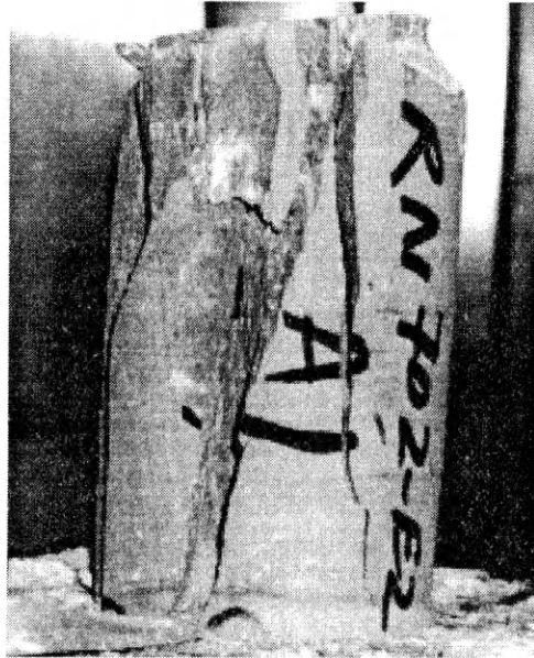
Figure 53: Typical non-structural sample failure for UCS testing
