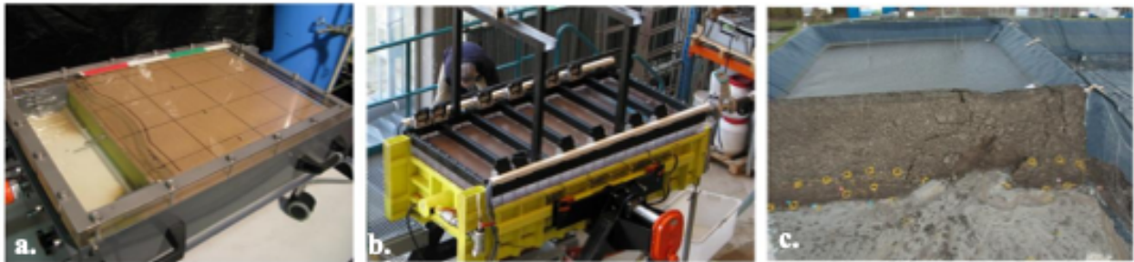
Figure 2.4. Illustration of (a) small scale experiments (0.8m length), (b) medium scale experiments (1.6 m seepage length), and large scale experiments (15 m) (van Beek, 2015).
