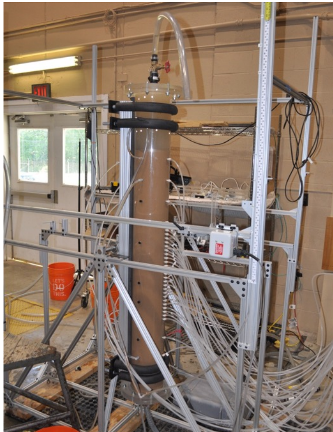
Figure 4.6. Photograph of cylindrical flume oriented vertically for sample preparation.
