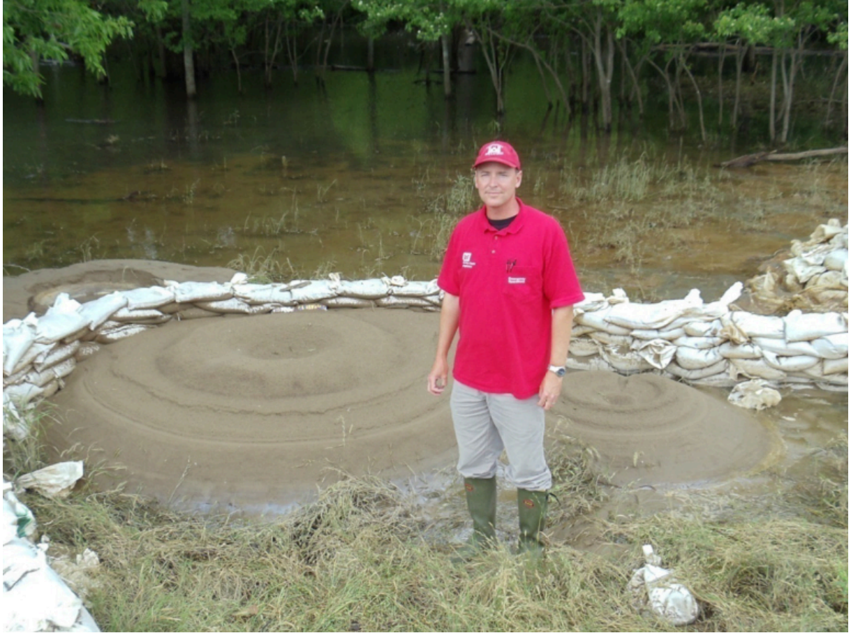
Figure 2.6. Large sand boils near Ensley Levee Memphis, TN during the 2011 Mississippi River Flood (Schaefer, et al., 2017)
