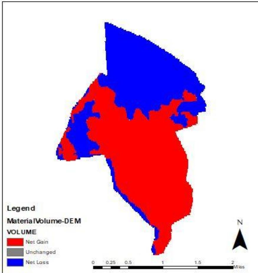
Figure 4.12: Cut and fill map (Blue area shows the cutting zone, red area shows filling zone). Cut volume = 163,157.56 ton: Fill volume = 642,184 ton
