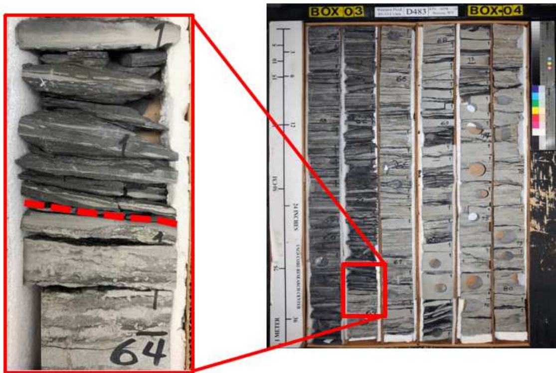
Figure 3.5: Core photo from the Colen 10-10 core displaying the Scaphites warreni flooding surface that is present throughout the subsurface and at the top of an upward coarsening sequence at 5,263-5,264 ft. core depth. Argillaceous mudstones overlying fine-grained sands can be observed at each FS within the Turner interval.
