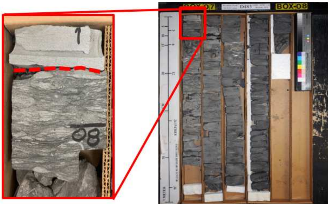
Figure 3.4: Core photo from the Colen 10-10 core displaying the Mid-Turonian unconformity (red dashed line) with the underlying Poole Creek member of the Carlile Shale at 5,307-5,308 ft. core depth.
