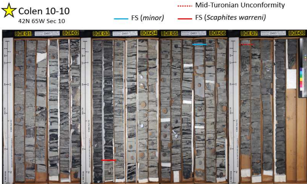
Figure 3.3: Core photos from the Colen 10-10 core displaying the Mid-Turonian unconformity (red dashed line) with the underlying Poole Creek member of the Carlile Shale at 5,307-5,308 ft. core depth. A minor flooding surface (blue solid line) with a medium- to fine-grained sandstone underlying a mudstone bed. at 5296-5297 ft. core depth. And a major flooding surface (red solid line) with a fine sandstone underlying an mudstone at 5263-6264 ft. core depth, capping the top of a Turner deposition cycle.
