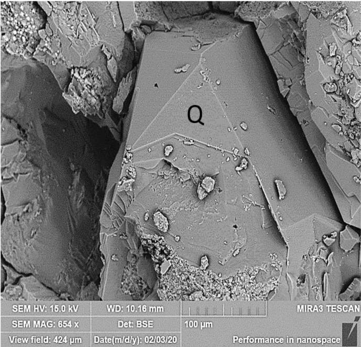
Figure 4.7: FE-SEM BSE image from the Colen 10-10 core at 5300 ft. core depth. BSE image shows a large euhedral quartz overgrowth (Q) in the pore space.
