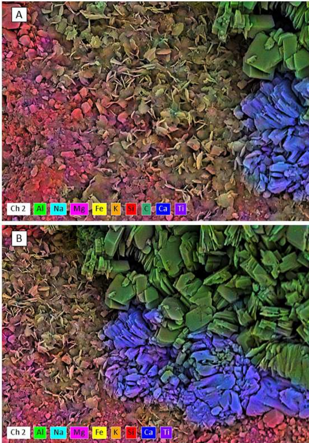
Figure 4.14: FE-SEM BSE image with EDS map from the Colen 10-10 core at 5297 ft. core depth. Authigenic microcrystalline quartz grain coat is shown in red, chlorite grain coat is seen in yellow, pore filling calcite cement is seen in blue, and pore filling authigenic kaolinite books are seen in green.
