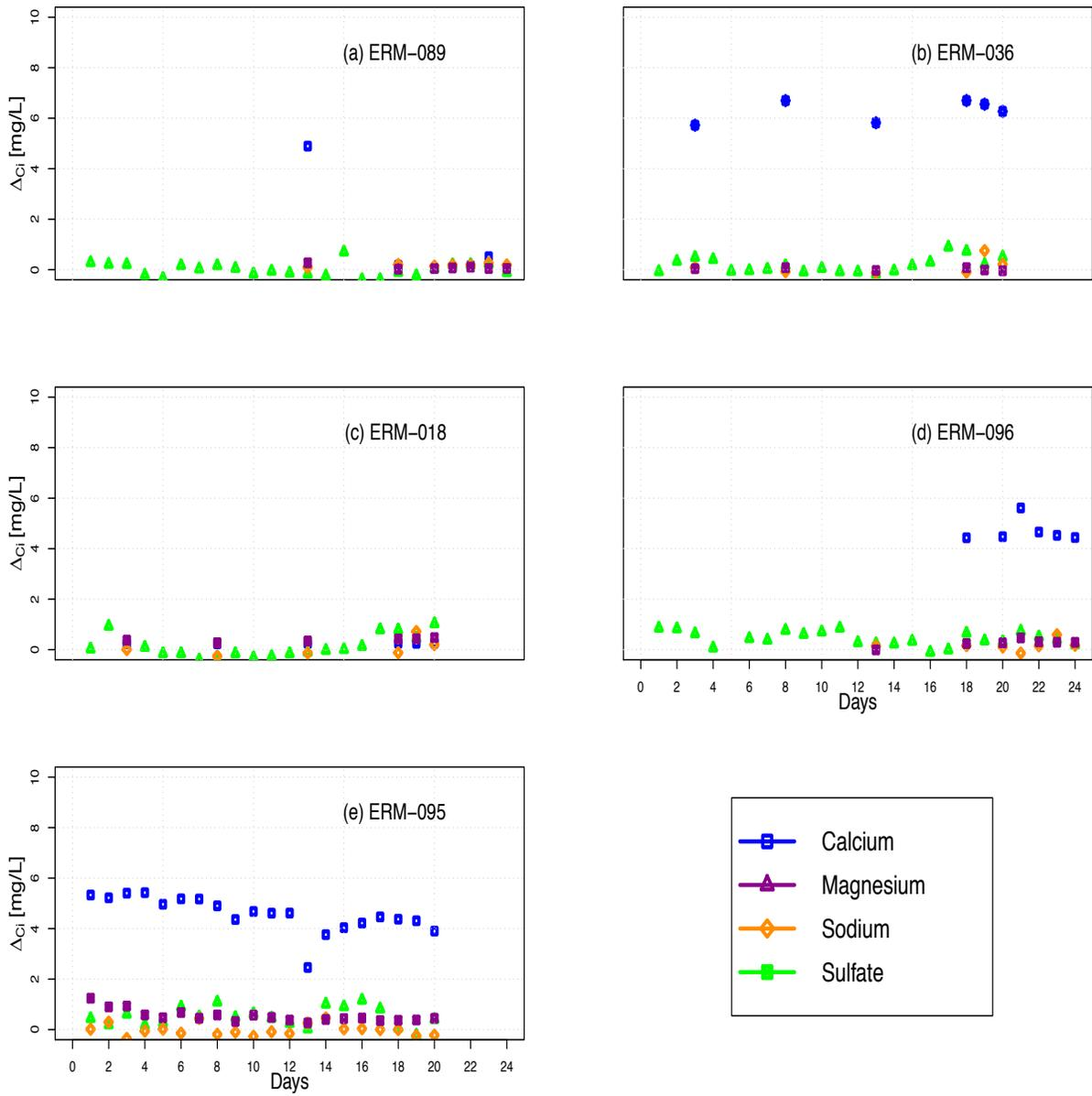
Figure 2.4  $\Delta C_i$  from IC data where  $\Delta C_i = C_{i(out)} - C_{i(in)}$  i represents analytes  $Ca^{2+}, Mg^{2+}, Na^+, SO_4^{2-}$
