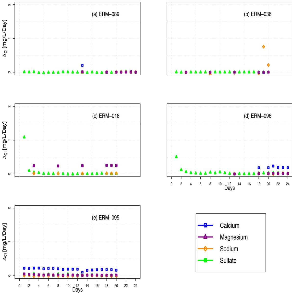
Figure 2.5  $\Delta C_i/\text{day}$  from IC data where  $\Delta C_i = C_{i(\text{out})} - C_{i(\text{in})}$   $i$  represents analytes  $\text{Ca}^{2+}$ ,  $\text{Mg}^{2+}$ ,  $\text{Na}^+$ ,  $\text{SO}_4^{2-}$ .
