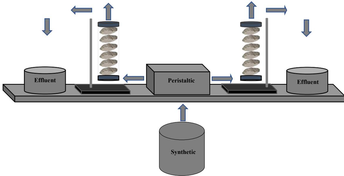
Figure 2.2 Conceptual Sketch of the flow through column experimental design.
