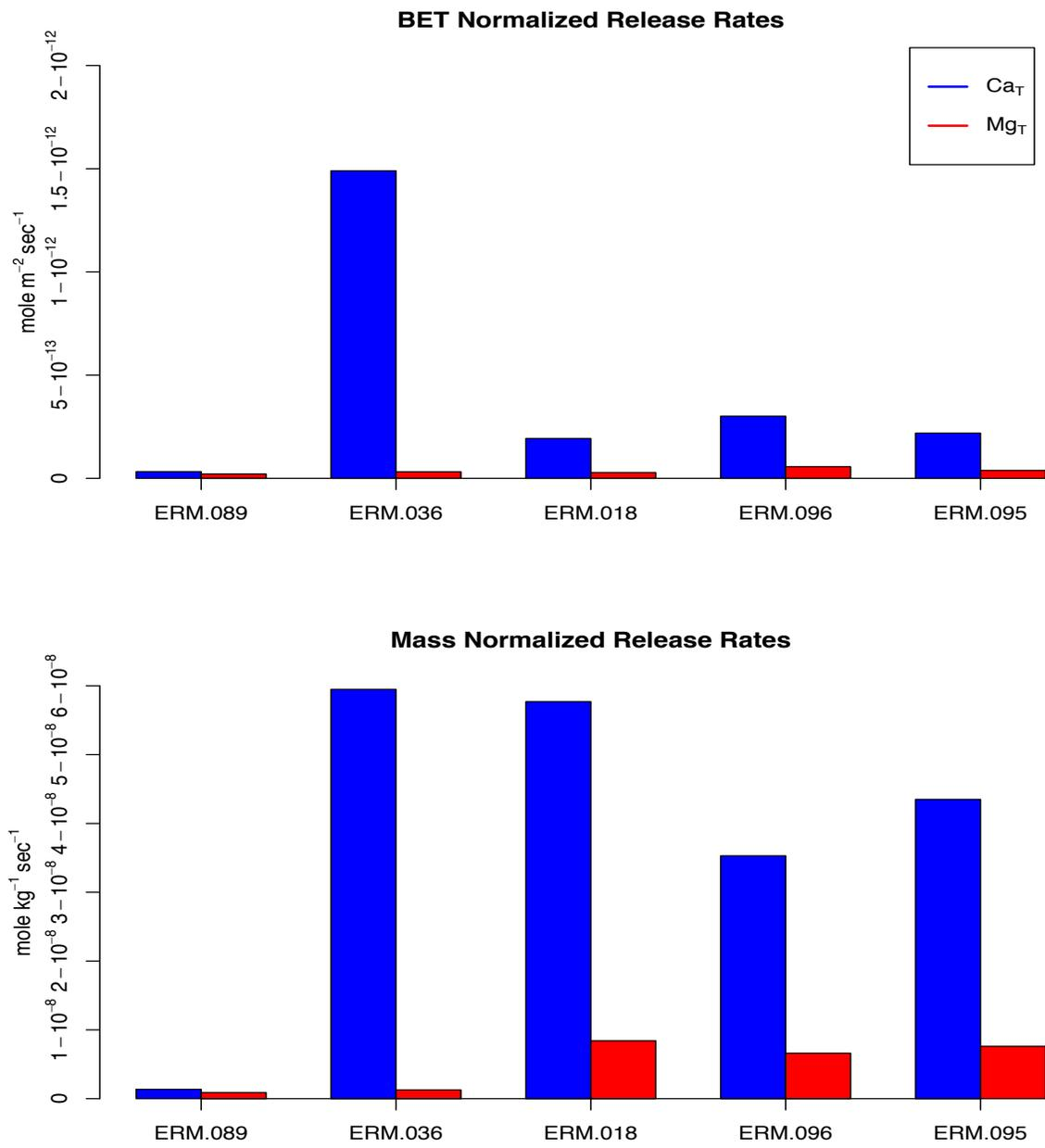
Figure 2.8 BET and Mass Normalized Rates for Ca<sub>T</sub> and Mg<sub>T</sub>. Data presented from most metamorphosed (left) to least metamorphosed.
