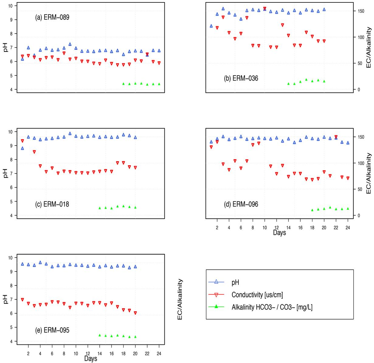
Figure 2.6 pH, conductivity and alkalinity data. Alkalinity data reported as HCO<sub>3</sub><sup>-</sup> for column ERM-089 because the pH ranges ≈ 6-7, where HCO<sub>3</sub><sup>-</sup> is the dominant carbonate species. Alkalinity data for all other columns reported as CO<sub>3</sub><sup>2-</sup> because the pH ranges ≈ 8-10, where CO<sub>3</sub><sup>2-</sup> is the dominant carbonate species.
