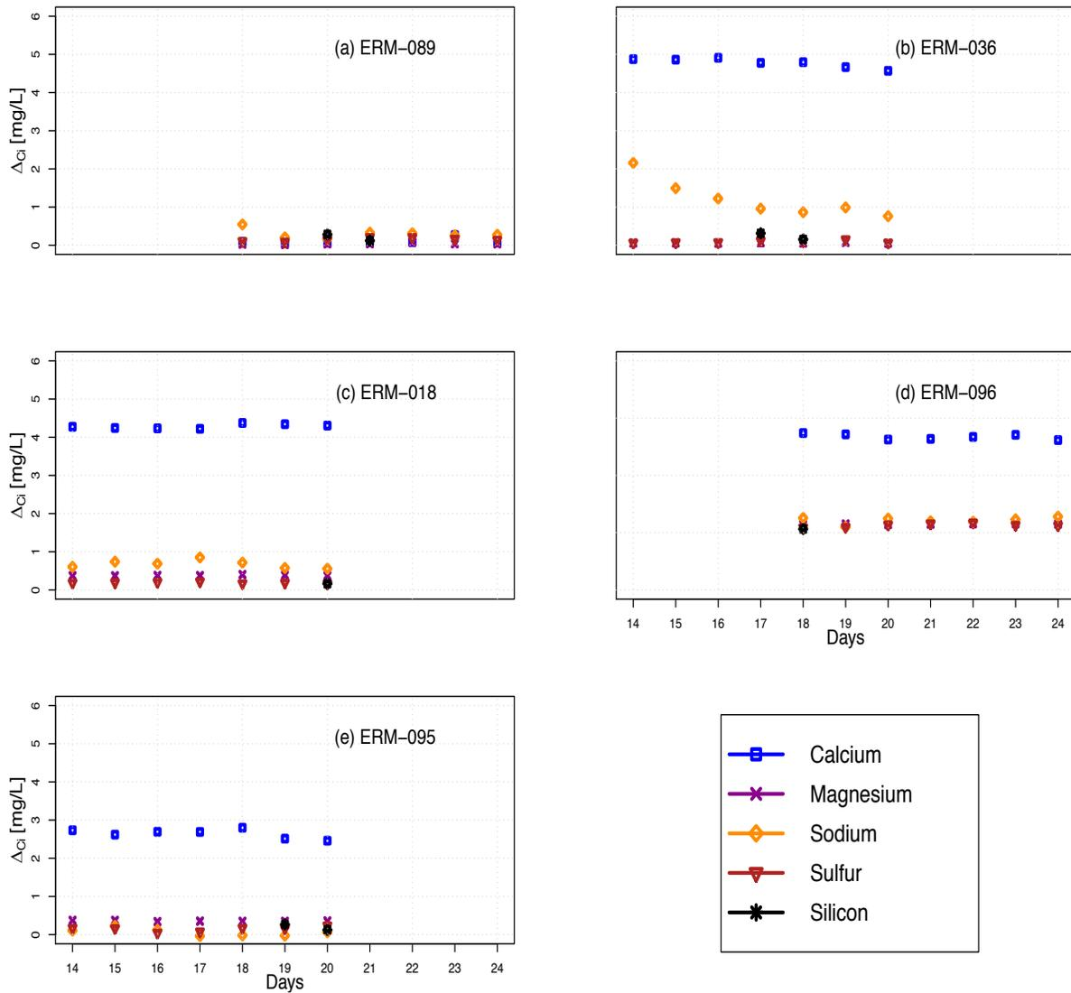
Figure 2.3 Steady state  $\Delta C_i$  where  $\Delta C_i = C_{i(out)} - C_{i(in)}$   $i$  represents analytes  $Ca_T$ ,  $Mg_T$ ,  $Na_T$ ,  $S_T$ ,  $Si_T$ .  $\Delta C_i$  used in steady state release rate calculations and normalized released rates.
