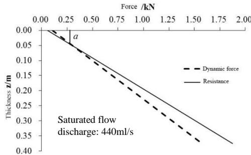
Fig. 3 The stress distribution of movable solid materials under saturated seepage flow
