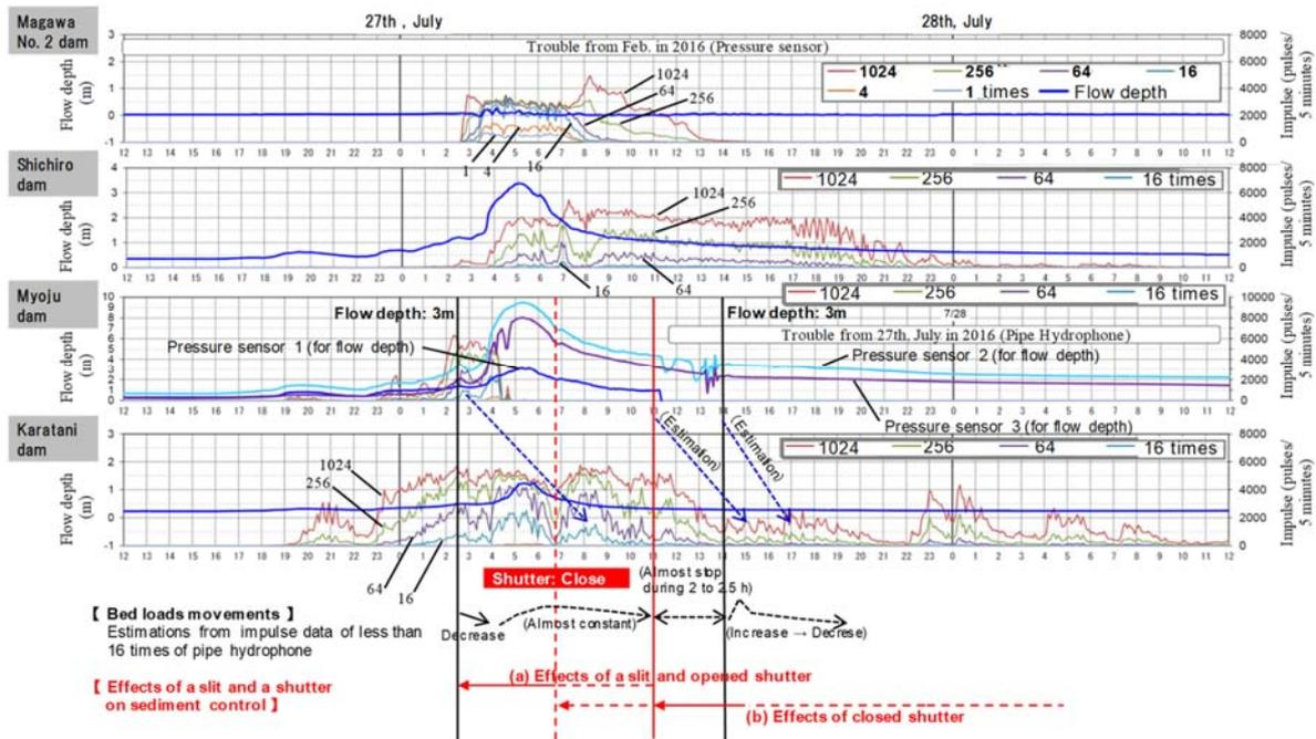
Fig. 8. Effects of shutter operation on longitudinal sediment transportation
