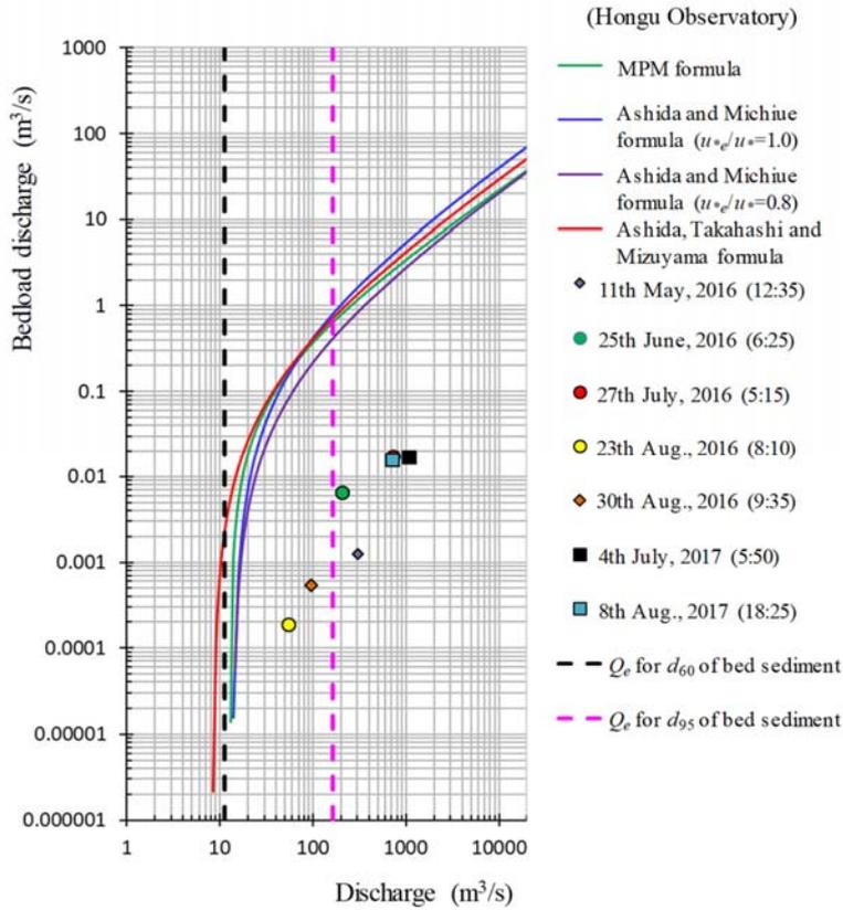
Fig. 4. Relationship between water discharge and bedload discharge
