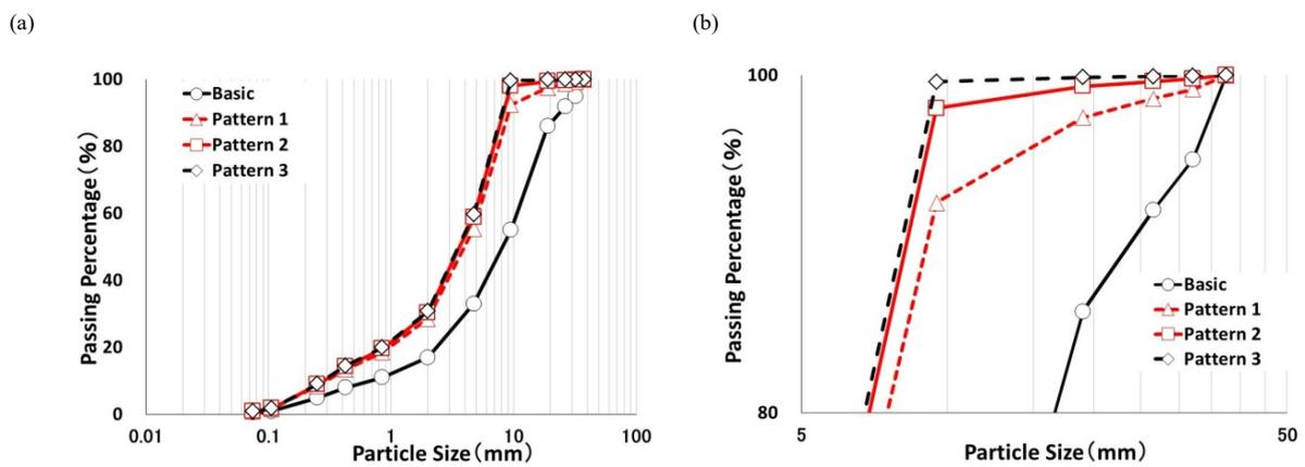
Fig. 4. (a) Particle size distribution of the main experimental sediment; (b) Particle size distribution enlarging 80-100%
