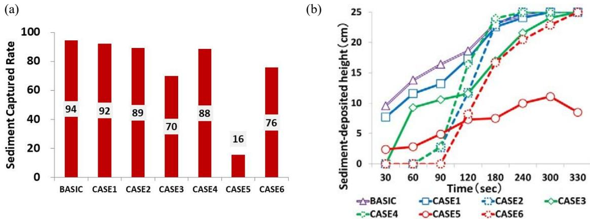
Fig. 5. (a) Sediment captured rate (Numbers in bars refer to the percent captured.); (b) Sediment-deposited height
