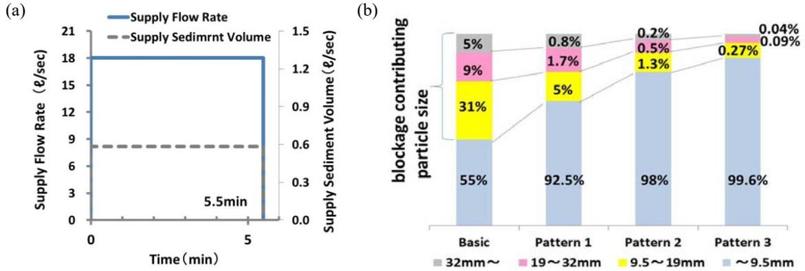
Fig. 3. (a) Hydrograph and sedigraph; (b) Particle size ratio
