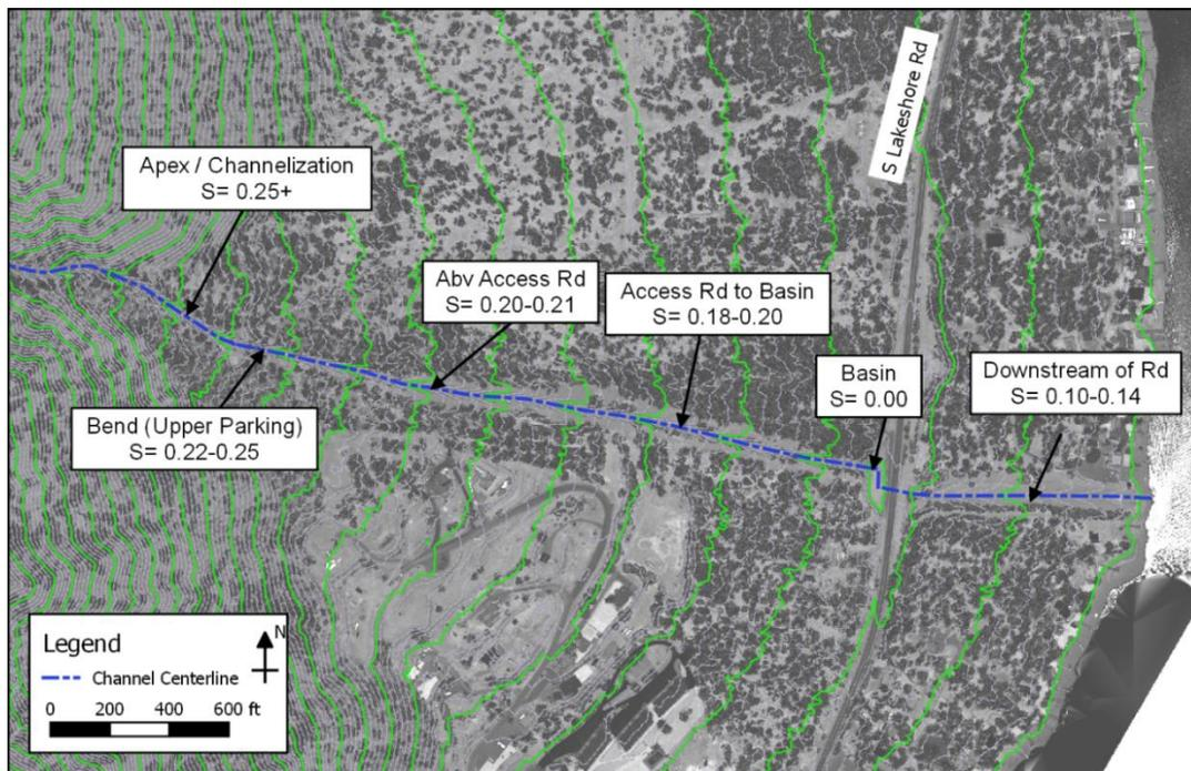
Fig. 1. Channel slopes based on 2018 Lidar for Slide Ridge debris channel.
