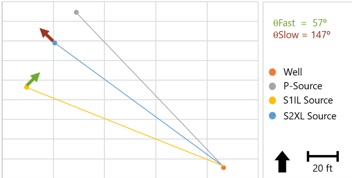
Figure 2.2 Map view of the pre-frac zero-offset VSP survey. The shaking directions of the shear sources are indicated by the red and green arrows. Lines are drawn connecting the source points to the well location (orange) to help visualize the different azimuths of the sources.
