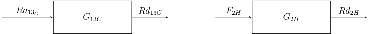
Figure 5.2: Schematic showing change in tracers in one compartment where Ra_{13C} is the rate of appearance of tracer I, F_{2H} is the infusion rate of tracer II and G is the accessible compartment of each tracer.
