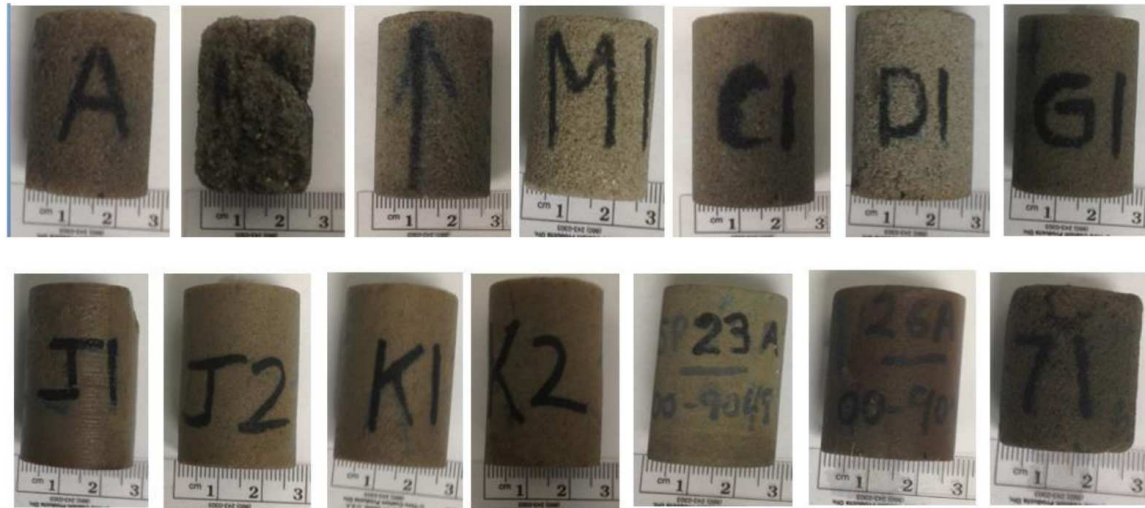
Figure 2.1: 14 core samples for Hibernia and Ben-Nevis formation. The samples have different colorization depending on the mineral composition, samples with lighter color have a high percentage of quartz. The images show different grain size distribution and cementation of the core which affect the pore space.
