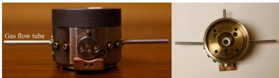
Figure 3.16 Assembling the diamond anvil cell for high temperature tests.
