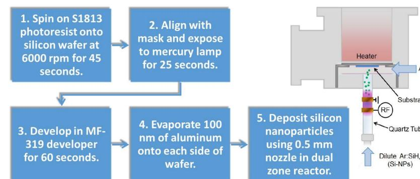
Fig. 5: Flowchart for fabricating quantum dot transistors (left) and diagram of dual zone reactor for growing nanoparticles (right) [2].
