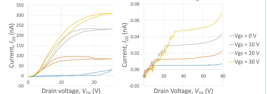
Fig. 8: Currents are orders of magnitude higher in the transfer characteristic of a nanocrystalline silicon transistor (left) than that of a silicon quantum dot transistor (right).
