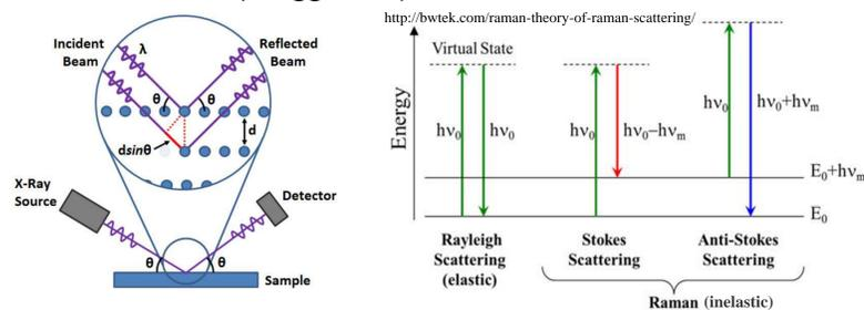
Fig. 1: Diagram of X-ray diffraction (left) [2] and energy diagram comparing Rayleigh and Raman scattering (right)
