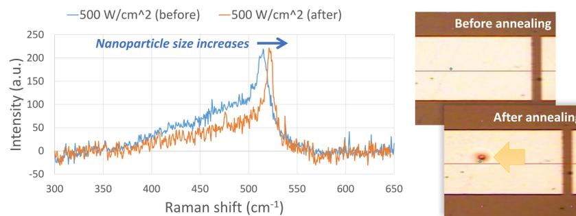
Fig. 3: Raman spectra (left) of silicon quantum dots before and after 5 minutes of exposure at  $50 \text{ kW/cm}^2$ ; laser-annealed spot is visible in optical microscope image (right)
