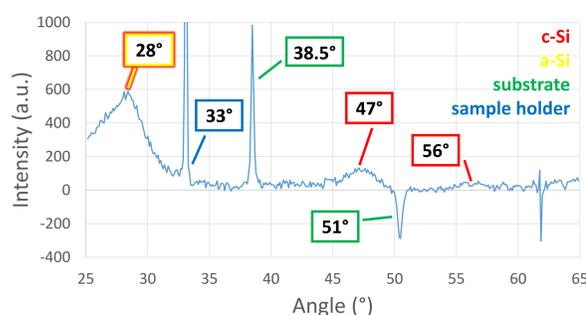
Fig. 2: Theta-two theta scan on silicon quantum dot thin-film transistors. Crystal silicon (c-Si) has peaks at 28°, 47°, and 56°. Amorphous silicon (a-Si) has peaks at 28°, 38°, and 52° [2]. The 38.5° peak is from aluminum in the substrate.
