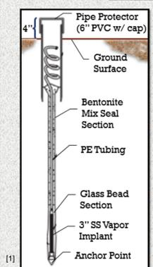
Manual Vapor Implant Soil Gas Sampler
