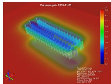
Figure 1: Model of reservoir with multiple wellbore trajectory and fractures
