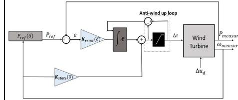
Figure 3. LPV Block Diagram with integral error reference tracking
