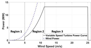
Figure 1. Operation Regions for a 13.2 MW variable speed wind turbine
