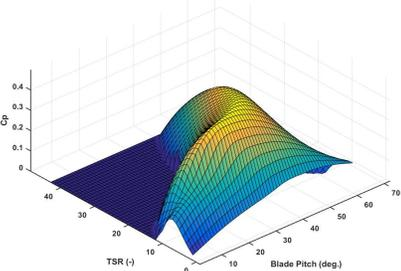
Figure 2.  $C_p$  Surface for the 13.2 MW SUMR.
