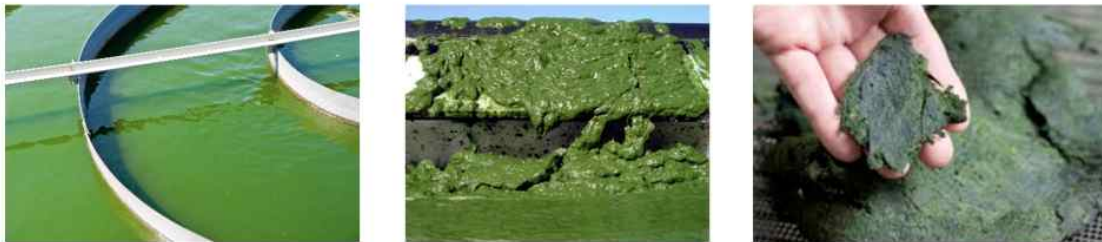
Figure 1.3. The concentration of microalgae cultures prior to lipid extraction. %TSS stands for total suspended solid. Pictured at bottom from left to right is the original algae effluent, followed by the algal slurry and then algal cake. Adapted from [18].
