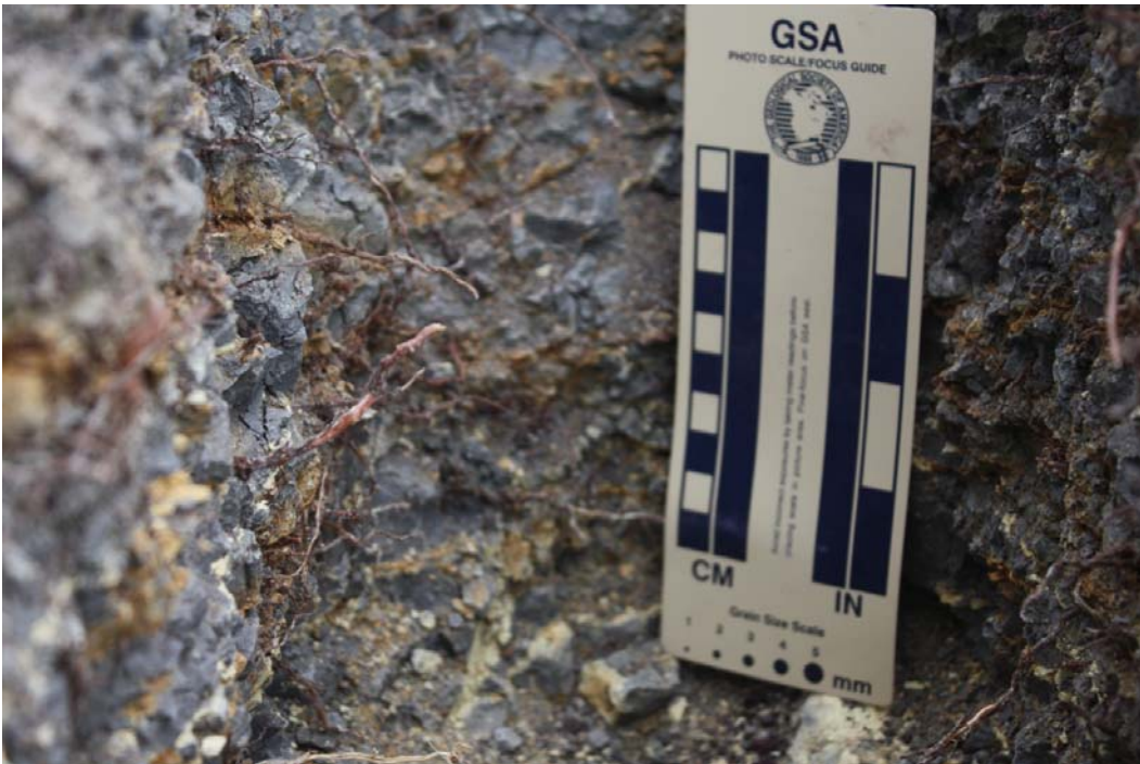
Figure 5.1.2.5a Close-up view of a paleosol from unit 10. Note the platy pedogenic texture, indicating some sedimentary structures are still present.
