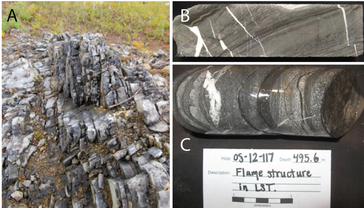
Figure B-6: Conrad limestone. A. Outcrop photo. Average bed thickness is around 4 cm. B. Drill core (NQ, ~4.8 cm diameter) photo with calcite veins oriented sub-perpendicular to bedding. C. Drill core (NQ) photo with flame structures.
