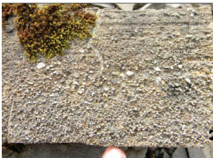
Figure B-15: Limestone grit. A. Hand sample photo with finger for scale. Note angularity of quartz granules
