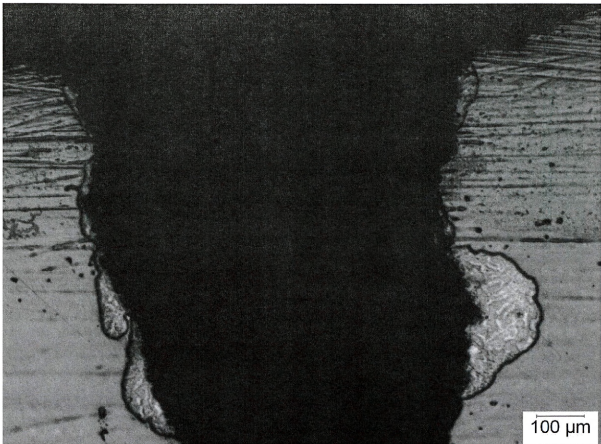
Figure 3.22 – Micrograph of brazed crack mouth. Remaining filler metal after partial emptying is evident in surface roughness on the crack surface.
