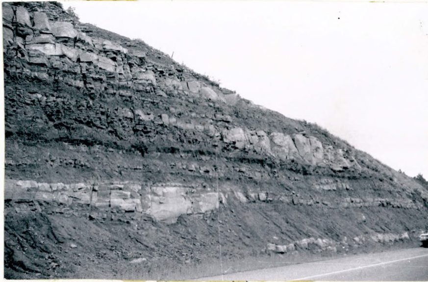
Figure 29. The lenticular sand pattern is common in a low energy environment of deposition (Unit No. 2), Raton Formation. Railroad Canyon.
