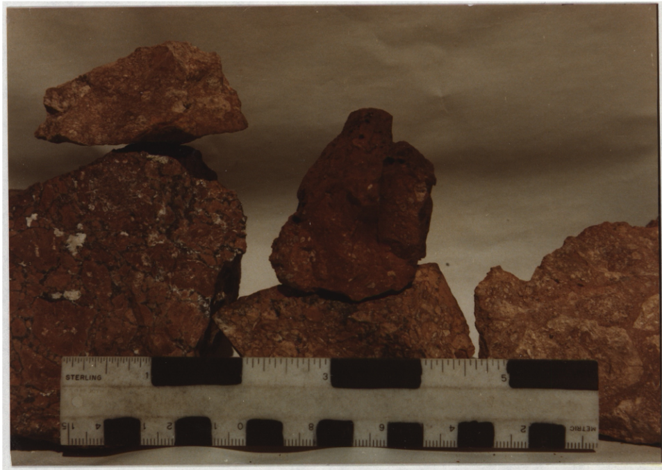
Figure 26. Hand samples of 'jasper rocks' formed by silicic alteration. Faint relict dacite-porphyry textures are visible in the less altered centers of breccia fragments. The breccia matrix is usually also dark silica, but may be specular hematite as seen in the lower left sample.
