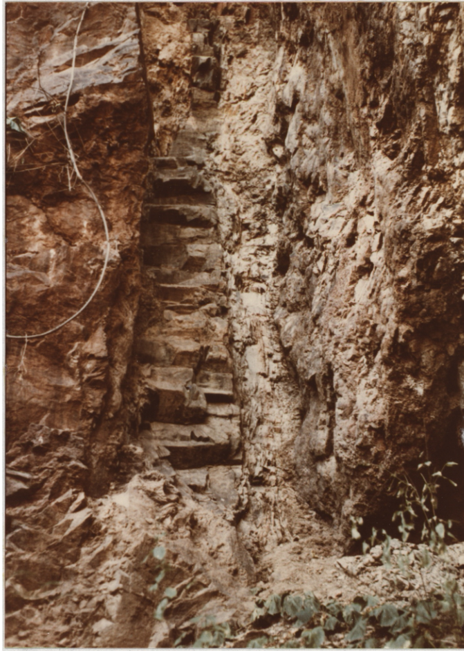
Figure 13. Basalt Dike exposed in old workings of the San Francisco mine. The dike is 1 m wide with horizontal columnar jointing. The right side of the dike is altered and friable, which in the workings below, is shown to result from calcite and zeolite saturation.
