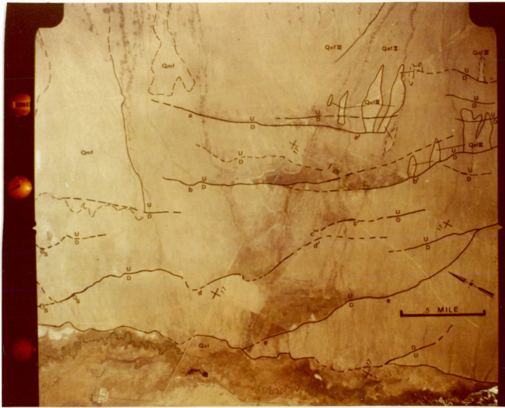
Figure 21a. Annotated reproduction of Mission 105 color photograph. Portion of Area 'A' shown. Qmf = mud flow; Qal = alluvium; Qaf II = fan Unit II; Qaf III = fan Unit III; Os = spring.
