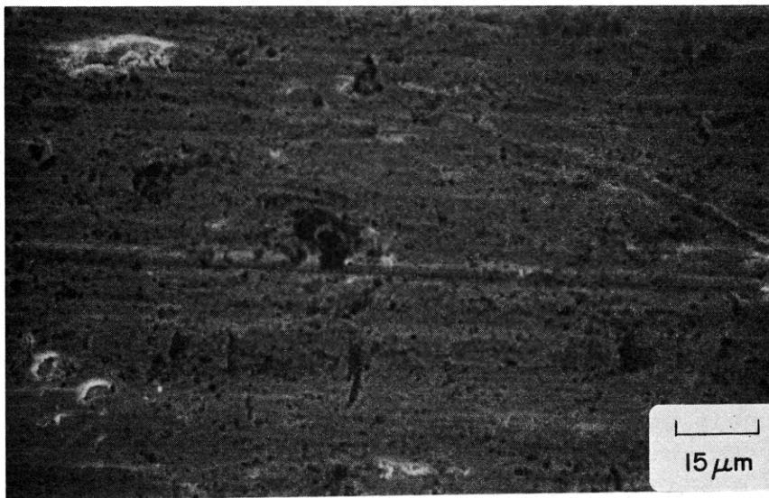
Figure 31. - SEM micrograph of wear scar of alloy 3.
