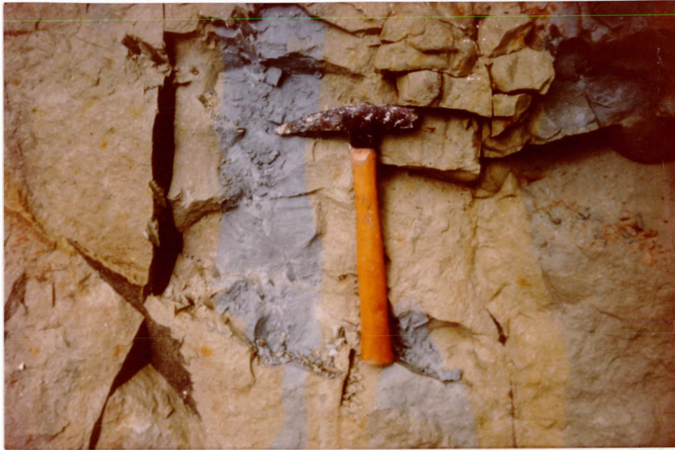
Figure 24. Massive muddy sandstone. Weathering progressing along fracture planes causes the alternance of bluish and brown coloration.
