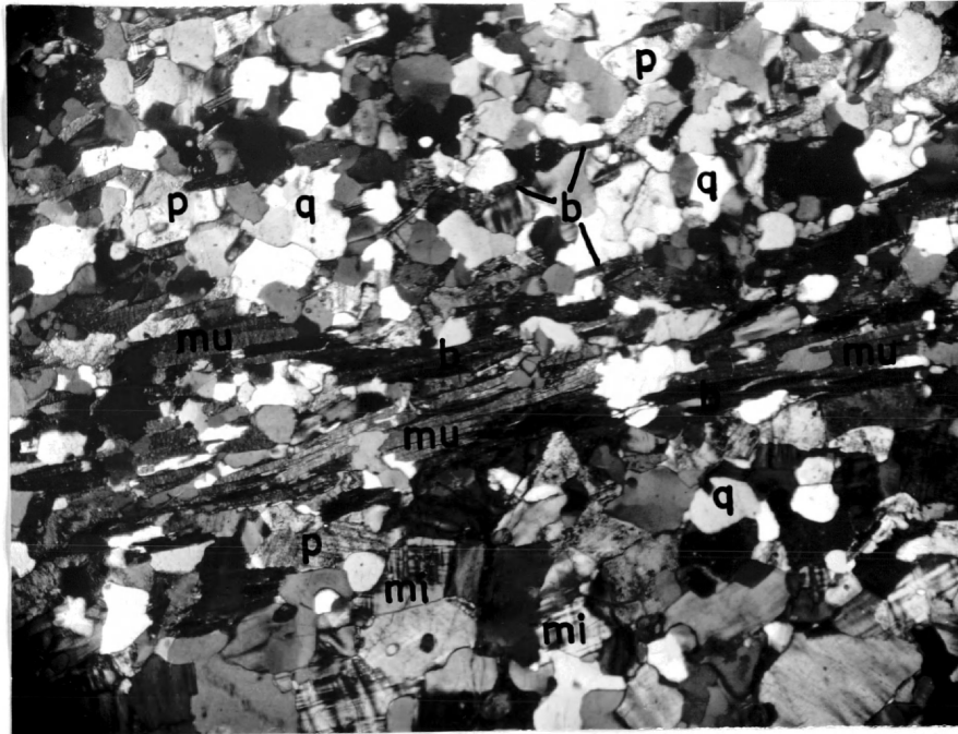
Figure 15: Photomicrograph of biotite-microcline-plagioclase-quartz gneiss from Phantom Canyon, sample PRC-27-71. mu-muscovite, b-biotite, mi-microcline, p-plagioclase, q-quartz. Crossed nicols, X25.
